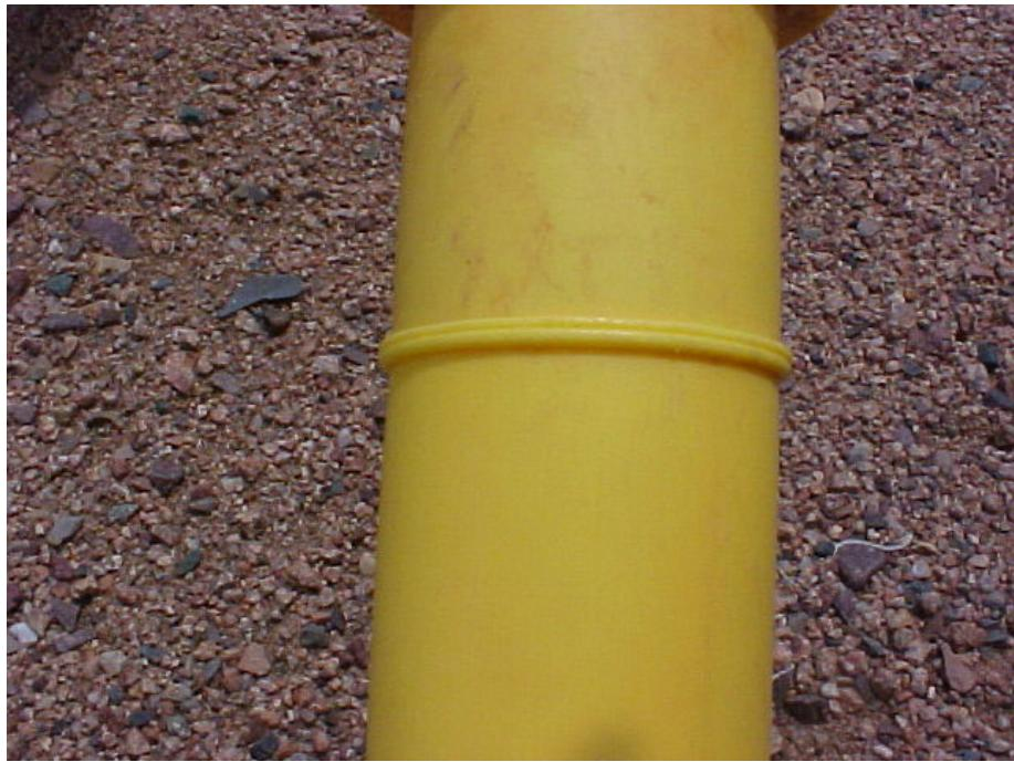
Fusion Butt Joint on plastic gas pipe.
