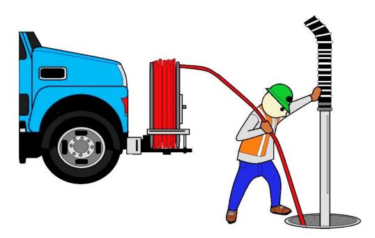
USING A VACUUM TRUCK TO CLEAN SEWER
