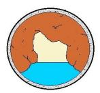
OVER TIME, THE BUILD-UP INCREASES WHEN GREASE AND DEBRIS ARE WASHED DOWN A DRAIN.
