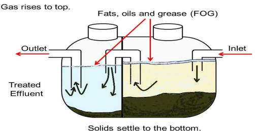
Diagram of a two-compartment grease interceptor's operation.
