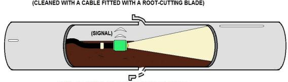
ROOT INTRUSION (CLEANED WITH A CABLE FITTED WITH A ROOT-CUTTING BLADE)
