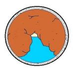
EXCESSIVE ACCUMULATION RESTRICTS THE FLOW OF WASTEWATER THAT CAN RESULT IN AN OVERFLOW OF SANITARY SEWER
