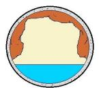
THE START OF BLOCKED PIPE BEGINS WITH SOLIDS AND GREASE COLLECTING ON TOP AND SIDES OF PIPE INTERIOR.
