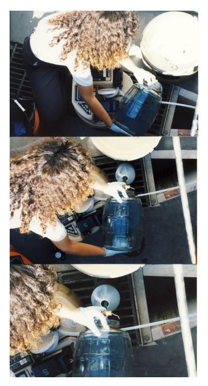
In this photo, you can see an automatic sampler and a pickle jar which are commonly used in a pretreatment program. The Inspector is pouring off a composite FOG sample for compliance testing. pH sampling is essential for a proper wastewater sampling program.
