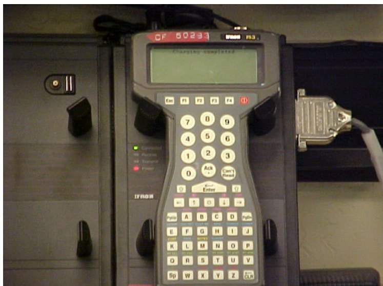
Computerized handheld electronic meter reader “station”
