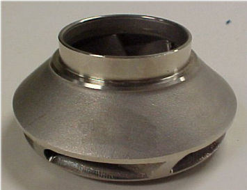
Below - A Small Closed Pump Impeller
