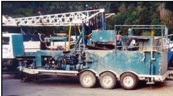
Small Self-Contained Mud System
