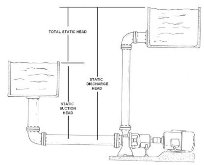
measurement does not take into account the friction caused by water moving through the hose or pipes. Dynamic indicates that losses due to friction are factored into the performance. The following terms are usually used when referring to lift or head.
