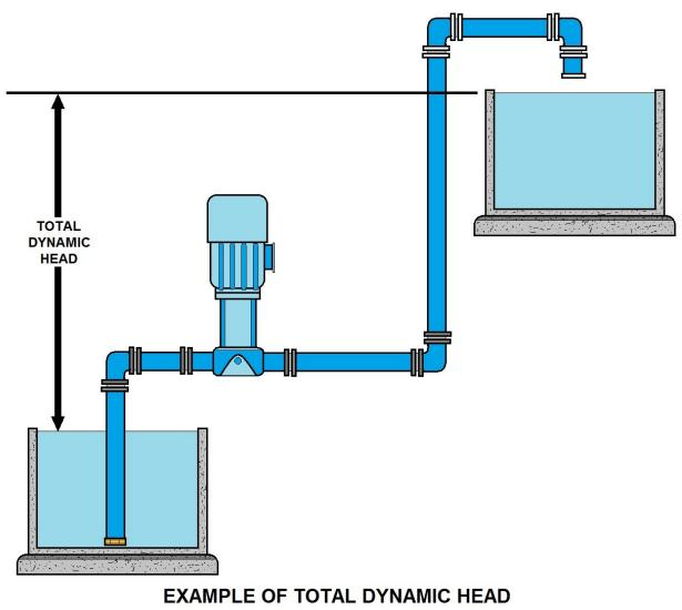
(The total equivalent height that fluid is to be pumped)
