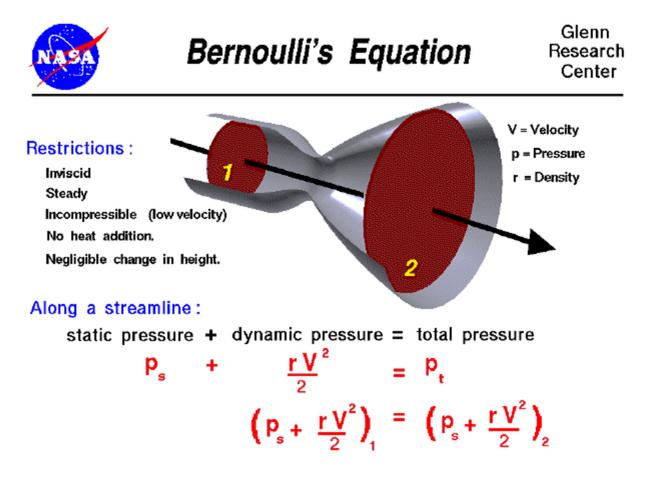
Here is where Bernoulli's equation figures in. As the water slows down and its kinetic energy decreases, that water's pressure potential energy increases (*to conserve energy*). Thus, the slowing is accompanied by a pressure rise. That is why the water pressure at the outer edge of the numer beauting is bighter than the
