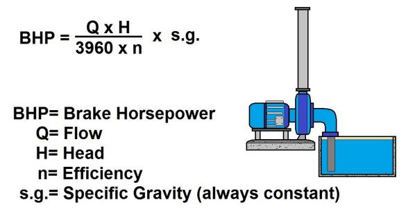
BRAKE HORSEPOWER (The available power of a motor assessed by measuring the force needed to brake motor)
