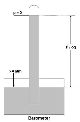
Suppose a vertical pipe is stood in a pool of water, and
