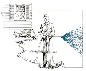
due to the higher speed of the air, which subsequently draws the fluid up. This is illustrated in the following figure.
