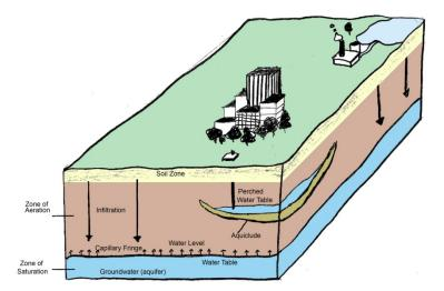
Groundwater usually flows downhill with the slope of the water table. Like surface water, groundwater flows toward, and eventually drains into, streams, rivers, lakes and the oceans.
