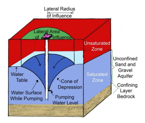
When a well is installed in an unconfined aquifer, water moves from the aquifer into the well through small holes or slits in the well casing or, in some types of wells, through the open bottom of the well. The level of the water in the well is the same as the water level in the aquifer. Groundwater continues to flow through and around the well in one direction in response to gravity.
