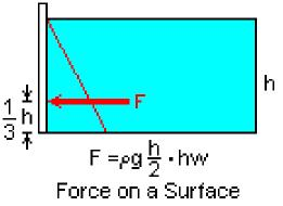
integral of  $dM' = \rho gxy dA$ , the moment about some vertical line in the plane of the surface.
