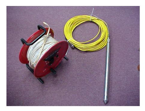
Groundwater Transducer (pH, Temp. chemical detection and D.O.) depth probe. These tools are used to find the depth and pH of well water.
