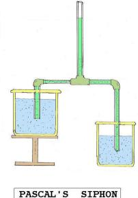
A siphon can be made by filling the tube, closing the ends, and then putting the ends under the surface on both sides. Alternatively, the tube can be placed in one fluid and filled by sucking on it. When it is full, the other end is put in place. The analysis of the siphon is easy, and should be obvious.
