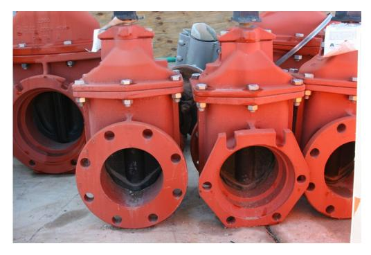
Gate valve storage procedures: Always store a gate valve with the gate up or opened. Not like in this picture. Sunlight will give these rubber components a good shot of Vitamin D and sunburn, destroying the rubber.
