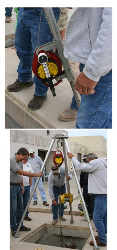
Checking the cable tension and inertial locking mechanism of the retrieval assembly.
