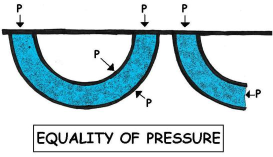
A fluid, therefore, is a substance that cannot exert any permanent forces tangential to a boundary. Any force that it exerts on a boundary must be normal to the boundary. Such a force is proportional to the area on which it is exerted, and is called a pressure.
