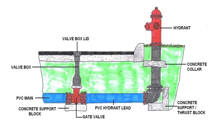
The above diagram is for proper fire hydrant and isolating gate valve installation. The diagram below represents how rust and electrolysis creates a hole or break in iron based water mains.
