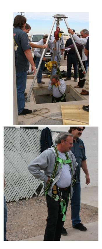
Dramatic rescue simulation using the tripod-retrieval system.
