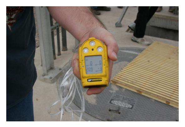
Here is a small clip-on style multi-purpose gas meter. We tied a string to lower the meter in the confined space to get a gas reading before entering.
