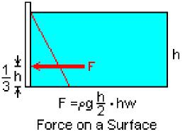
integral of  $dM' = \rho gxy dA$ , the moment about some vertical line in the plane of the surface. If there happens to be a pressure on the free surface of the water, then the forces due to this pressure can be evaluated separately and added to this result. We must add a force equal to the area of the surface times the additional pressure, and a moment equal to the product of this force and the distance to the centroid of the surface.
