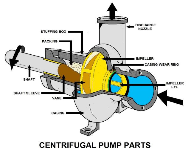
As the impeller rotates, it sucks the liquid into the center of the pump and throws it out under pressure through the outlet. The casing that houses the impeller is referred to as the volute, the impeller fits on the shaft inside. The volute has an inlet and outlet that carries the water as shown below.
