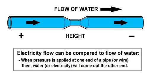
(Flow of electrons (electricity) along a wire)
