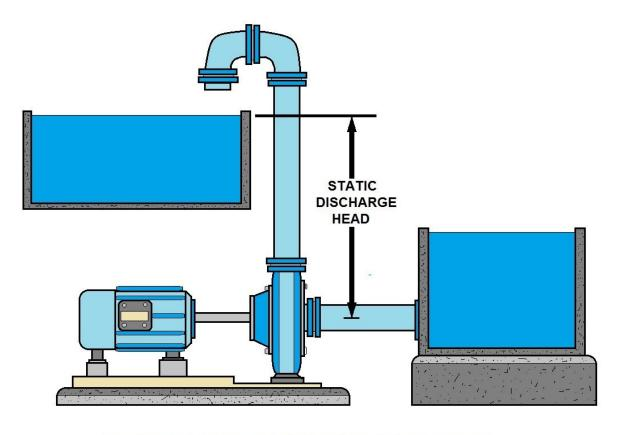
EXAMPLE OF STATIC DISCHARGE HEAD (The vertical distance from discharge outlet to point of discharge)
