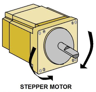
Brushless, Synchronous Electric Motor that coverts digital pulses into shaft rotations
