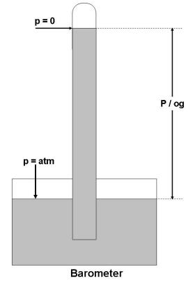
Suppose a vertical pipe is stood in a pool of water, and a vacuum pump applied to the upper end. Before we start the pump, the water levels outside and inside the pipe are equal, and the pressures on the surfaces are also equal and are equal to the atmospheric pressure.
