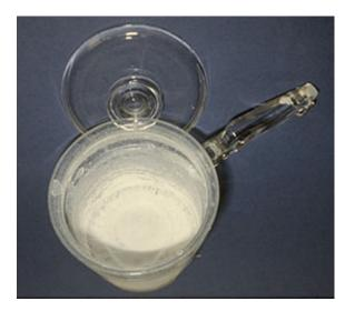
When hard water is heated, scale forms much faster. In particular, when the magnesium hardness is more than about 40 mg/l (as  $CaCO_3$ ), magnesium hydroxide scale will deposit in hot water heaters that are operated at normal temperatures of 140-150°F (60-66°C).
