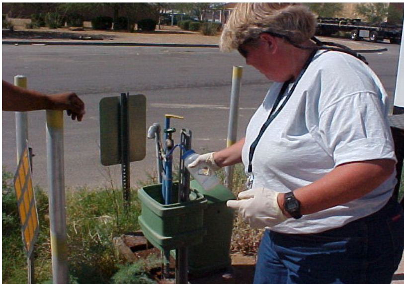
Using alcohol to disinfect a special sample tap before obtaining a sample.
