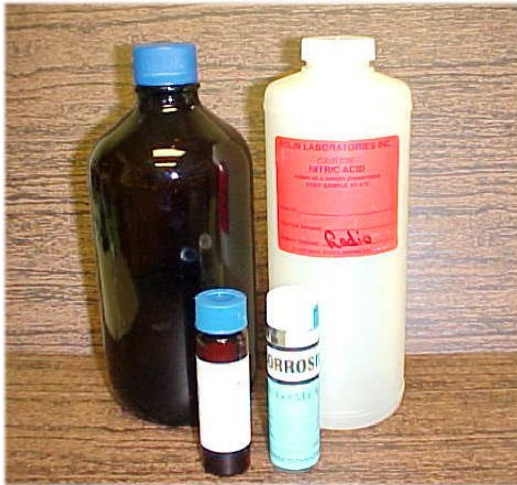
Common water sample bottles for distribution systems.
