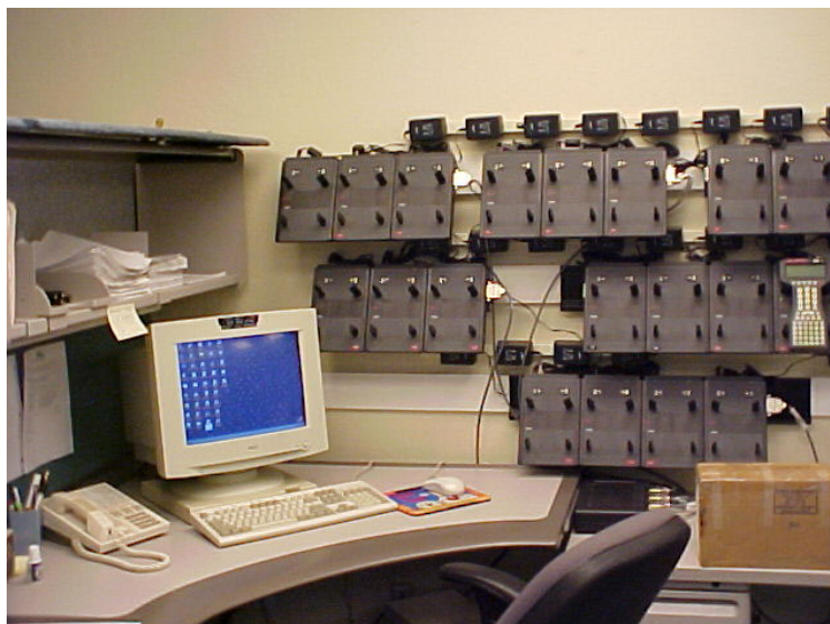
Computerized handheld electronic meter reader “station”
