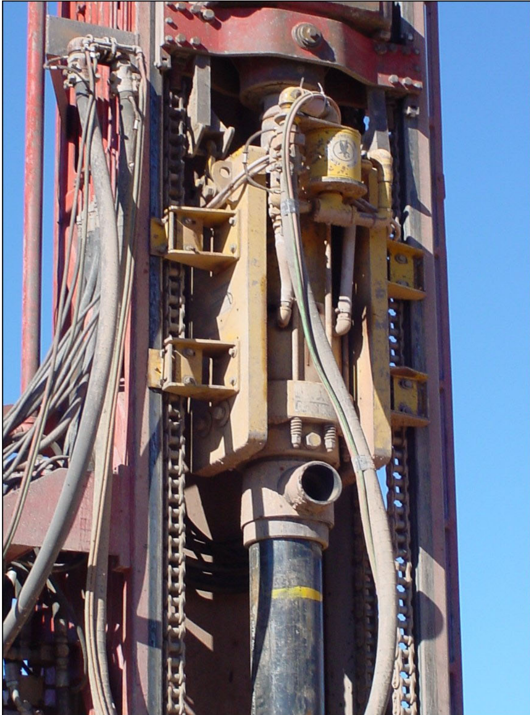
A Casing Driver attached to a top drive air rig.
