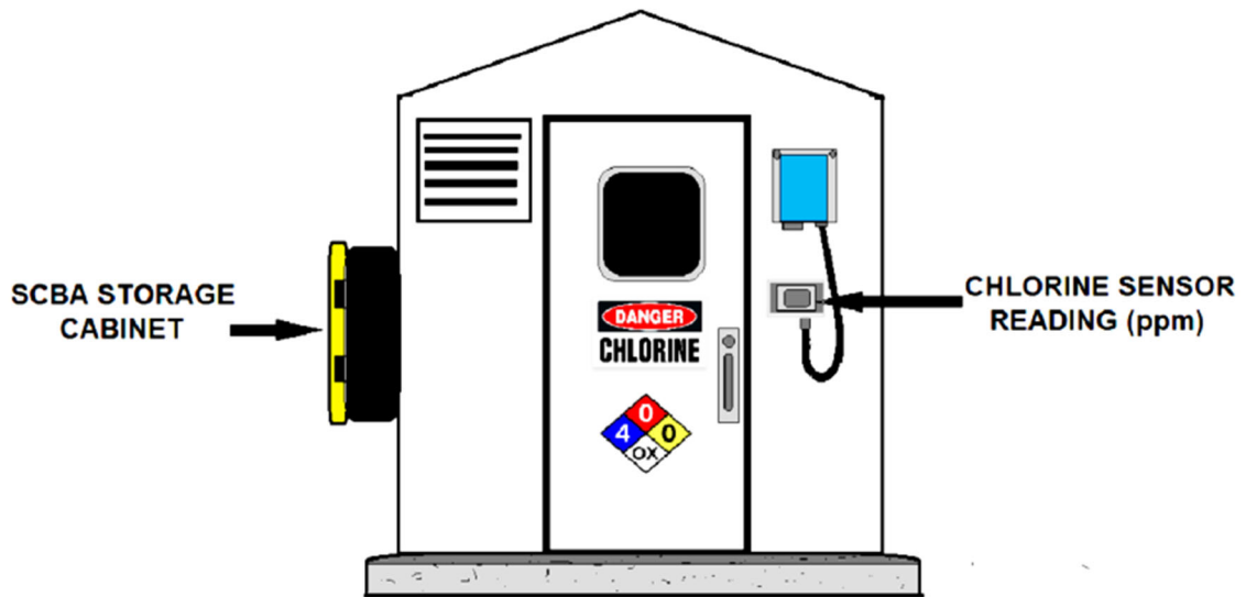
FIBERGLASS CHLORINE STORAGE SHELTER
