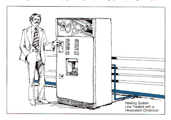
Several cross-connection have been made to soda machines, the one to worry about is when you have a copper water line hooked to CO<sub>2</sub> without a backflow preventer.
