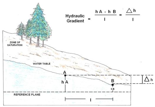
The *hydraulic gradient* is a vector gradient between two or more hydraulic head measurements over the length of the flow path. It is also called the 'Darcy slope', since it determines the quantity of a Darcy flux, or discharge. A dimensionless hydraulic gradient can be calculated between two piezometers as:
