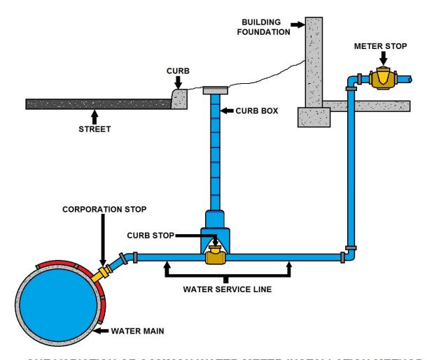
ONE VARIATION OF COMMON WATER METER INSTALLATION METHOD
