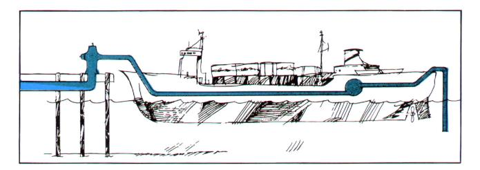
Here we see the backpressure of salt water back into the public water system from a ship's pressure pump. Most water providers are now requiring a RP assembly at the hydrant.
