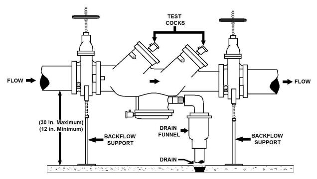
REDUCED PRESSURE BACKFLOW PREVENTER (Indoor Installation)
