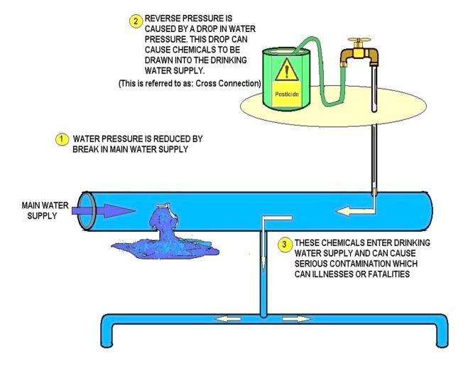
Above is one example of a commonly found cross-connection. This type pf cross-connection happens every time the water pressure in the water main is reduced or shutdown.
