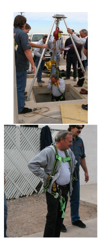
Dramatic rescue simulation using the tripod-retrieval system.
