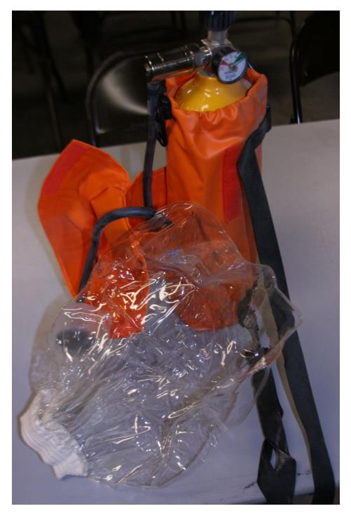
This is a ten-minute escape air pack or emergency air supply. The plastic bag with go over your head during an emergency and provide enough air to get out of the hole. There are smaller versions of this system.
