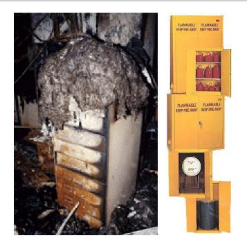
A fire resistant file cabinet that is burned completely and beside it are modern flammable liquids storage cabinets.
