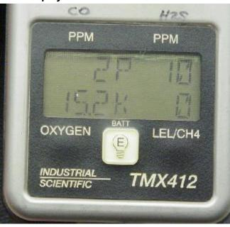
Example Display for Peak Mode: The display reads 2 ppm peak value for CO and 10 ppm peak value for H<sub>2</sub>S (top line);
