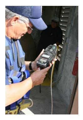
Checking the atmosphere with a gas meter is essential for entering any permit required confined space.
