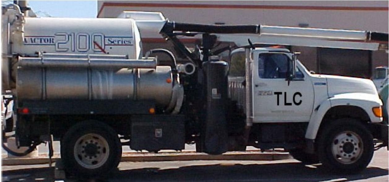
The sewer vacuum truck utilizes both a high pressure stream of water and a vacuum system to clean and remove built up debris from sewer lines. These versatile vehicles are also used to clean lift station wet wells, stormwater catch basins, and to perform excavations to locate broken water or sewer lines. It reduces repair times and costs by over 50%.
