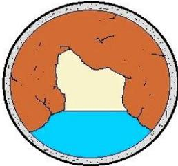
**OVER TIME, THE BUILD-UP INCREASES WHEN GREASE AND DEBRIS ARE WASHED DOWN A DRAIN.**
