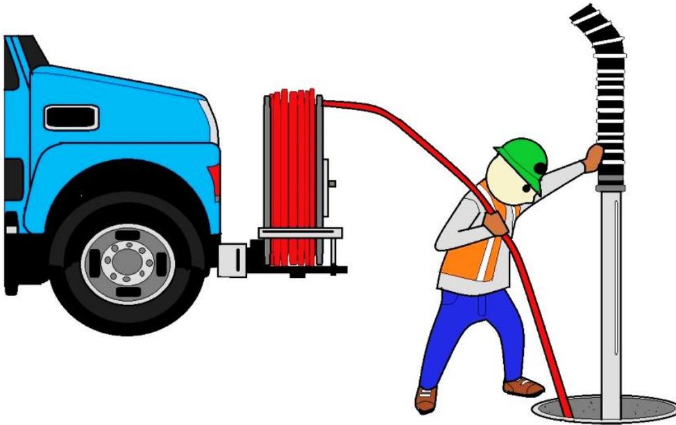
**USING A VACUUM TRUCK TO CLEAN SEWER**
