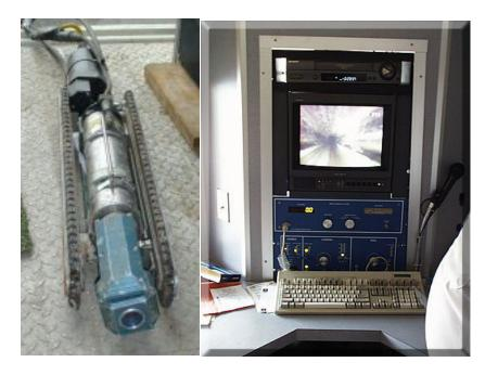
The Televising Van should be equipped with two cameras, one color camera for televising main sanitary lines and one color or black & white camera for televising house services (connection from the main sanitary line to a house).
