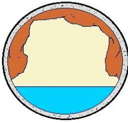
**THE START OF BLOCKED PIPE BEGINS WITH SOLIDS AND GREASE COLLECTING ON TOP AND SIDES OF PIPE INTERIOR.**
