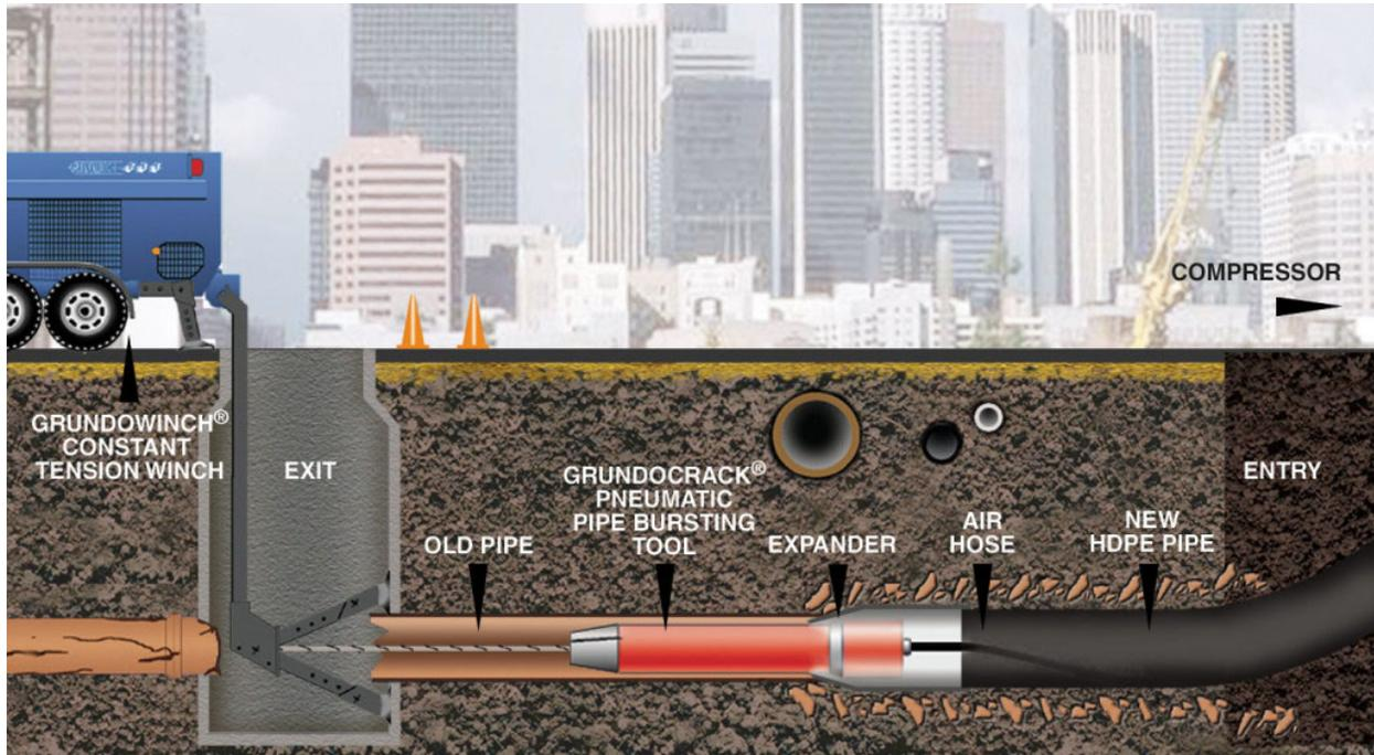
Cast iron and clay sewer lines often have more points of failure than high density polyethylene pipe or HDPE because they have more joints and joints. HDPE pipe is seamless, and so introduces fewer potential points of failure.
