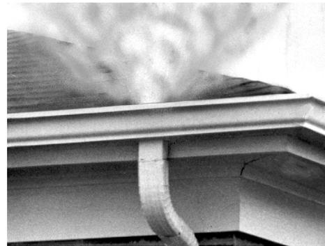
The smoke travels the path of least resistance and quickly shows up at sites that allow surface water inflow. Smoke will identify broken manholes, illegal connections (including roof drains, sump pumps, yard drains and more), uncapped lines, and will even show cracked mains and laterals providing there is a passageway for the smoke to travel to the surface.
