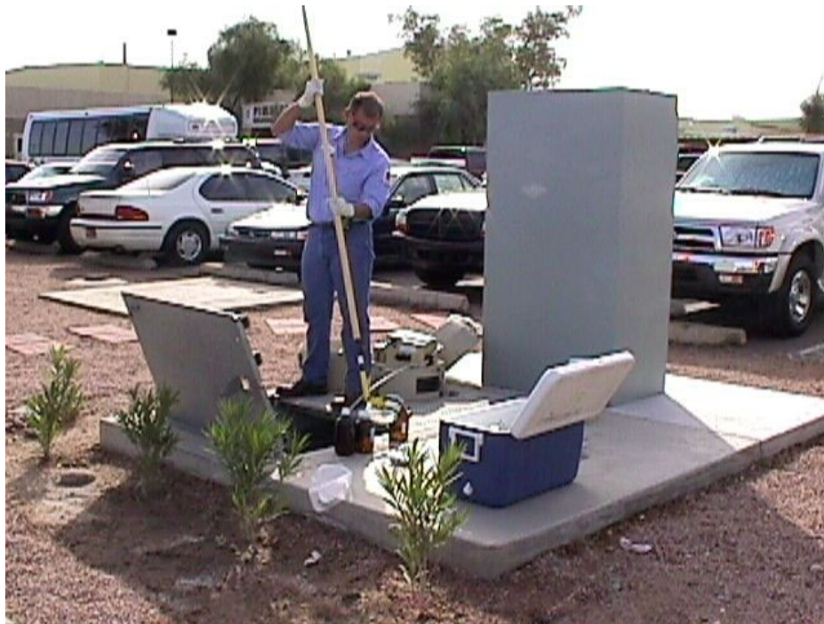
A Pretreatment Inspector sampling an SIU Interceptor. A great job promotion for any Collection System's Operator.
