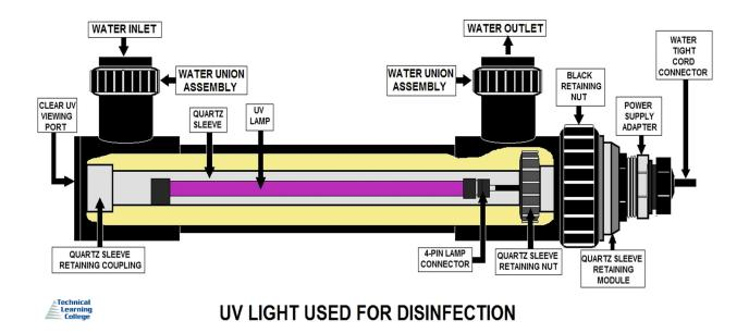
Ultraviolet light for disinfection was primarily used in the wastewater industry because of its effectiveness to deactivate microorganisms and not having to dechlorinate the effluent for discharge. In drinking water, UV has become popular because it doesn't produce Trihalomethanes however there is no residual disinfectant. Another consideration is the cost to operate and maintain the UV unit.
