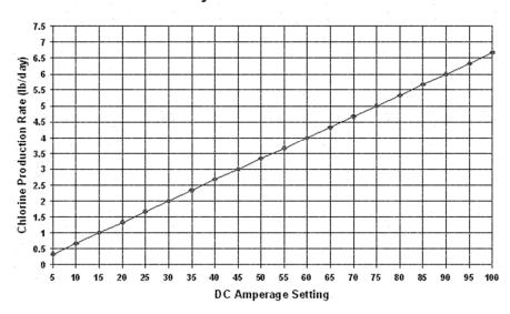
**Note:** With time, the membrane accumulates calcium and other mineral deposits that increase the resistance between the electrodes. The increased resistance causes a reduced amperage output and a corresponding reduced chlorine output. The system needs periodic membrane cleaning to recover the desired amperage output. A water softener system can be added to the system water supply to reduce the amount of calcium, thus increasing the service life of the membrane.
