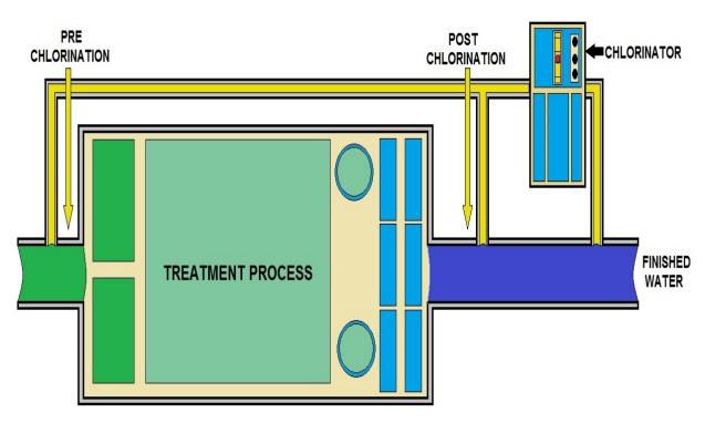
CHLORINE FLOW IN A TREATMENT PLANT DIAGRAM
