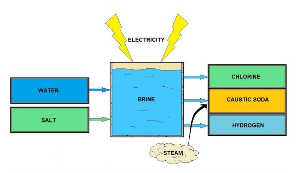
BASIC CONCEPT OF HOW CHLORINE AND CAUSTIC SODA ARE PRODUCED
