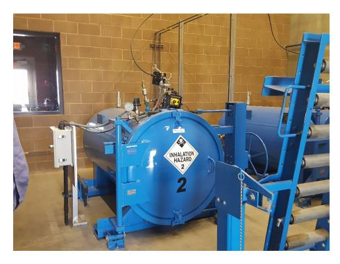
These photos are of high-pressure chlorine containment vessels into which a 1-Ton or 150-lb chlorine gas cylinder is processed. If the cylinder should leak, chlorine gas is contained within the vessel and processed at a normal rate. All of the chlorine gas is used and no hazardous waste is generated.
