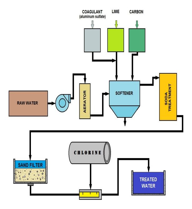
Water treatment plant chlorine addition diagram
