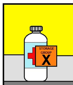
STORAGE GROUP X MUST BE SEGREGATED FROM ALL OTHER CHEMICALS
