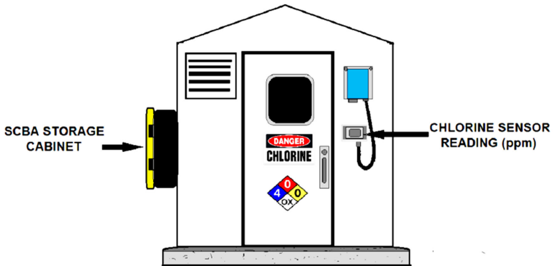
FIBERGLASS CHLORINE STORAGE SHELTER
