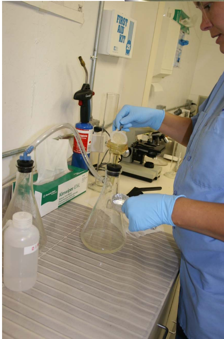
Lab tech removing filter for TSS analysis.
