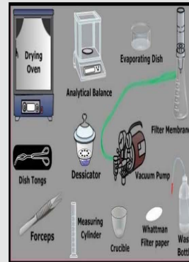
EQUIPMENT USED TO MEASURE AND DETERMINE TYPES OF SOLIDS
