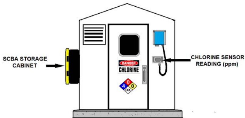
FIBERGLASS CHLORINE STORAGE SHELTER
