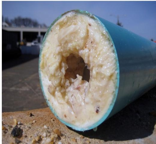
Wastewater onsite (septic) systems also can be harmed by too much fats, oil and grease, which can clog onsite system drainfield pipes and soils, adding to the risk of system failure. Excessive grease also adds to the septic tank's scum layer, causing more frequent tank pumping to be required. Both conditions can result in significant costs to homeowners.
