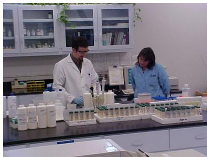
Two lab techs examine various samples, including QA/QC and Trip Blanks to ensure both sample integrity and lab equipment/sample equipment quality.
