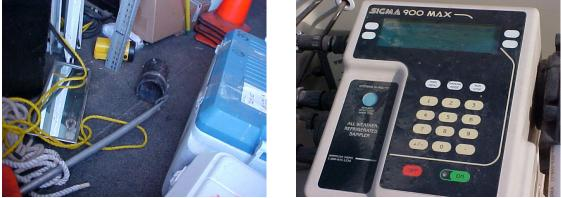
**Tools of the Trade**... Above photos, the refrigerated automatic sampler will have a Data programmer which will allow you to set the time to collect the sample or samples. This machine can also measure the amount of the sample.
