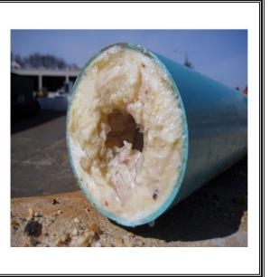
Wastewater onsite (septic) systems also can be harmed by too much fats, oil and grease, which can clog onsite system drainfield pipes and soils, adding to the risk of system failure. Excessive grease also adds to the septic tank's scum layer, causing more frequent tank pumping to be required. Both conditions can result in significant costs to homeowners.
