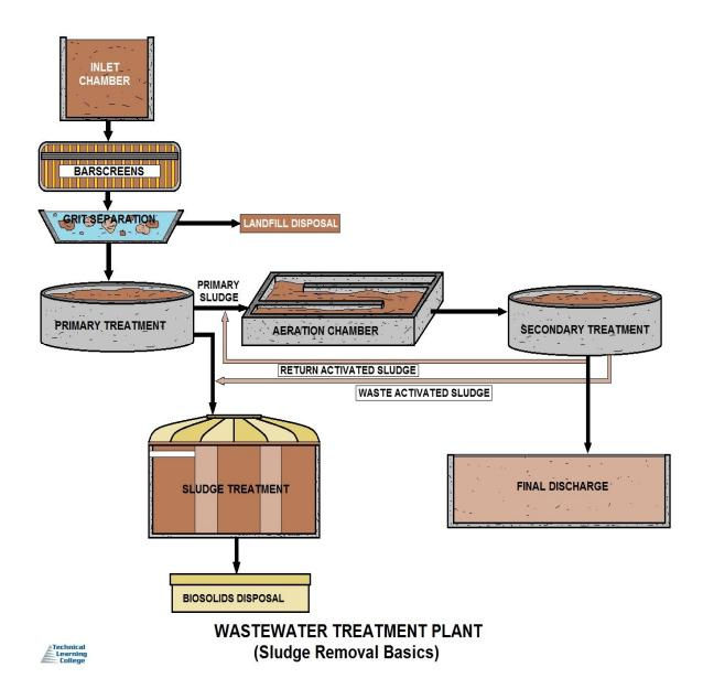
There are various options for treating sludge including stabilization, thickening, dewatering, drying, and incineration. The costs for treating sludge and removing sludge from wastewater are roughly the same. Typically a polymer chemical is used for the volume reduction process known as dewatering. Polymers are slippery chemicals, which means that there is always a risk of slipping or falling due to spills and leaks. Polymers can also be environmental stress crack agents.
