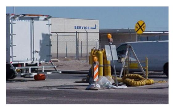
Wastewater sampler set-up in traffic to obtain composite sample from a sewer manhole. Notice the tri-pod and barricades.
