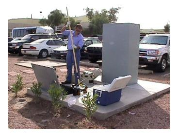
Using an extension pole with a sampling attachment to grab a sample.
