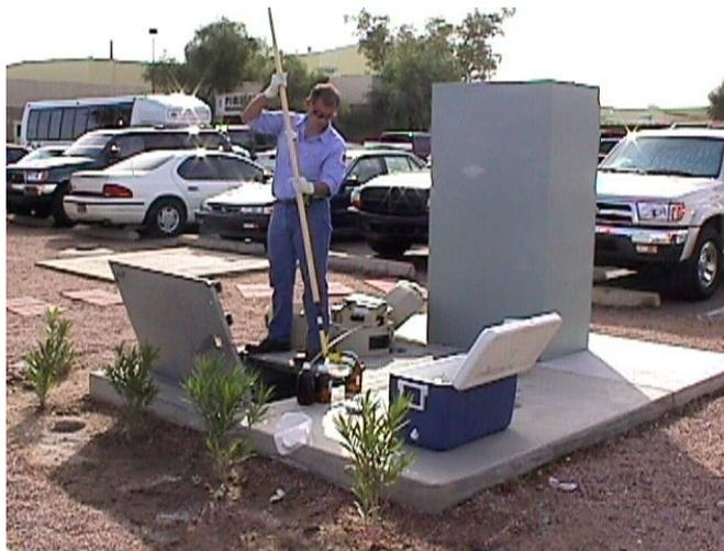
Using an extension pole with a sampling attachment to grab a sample.
