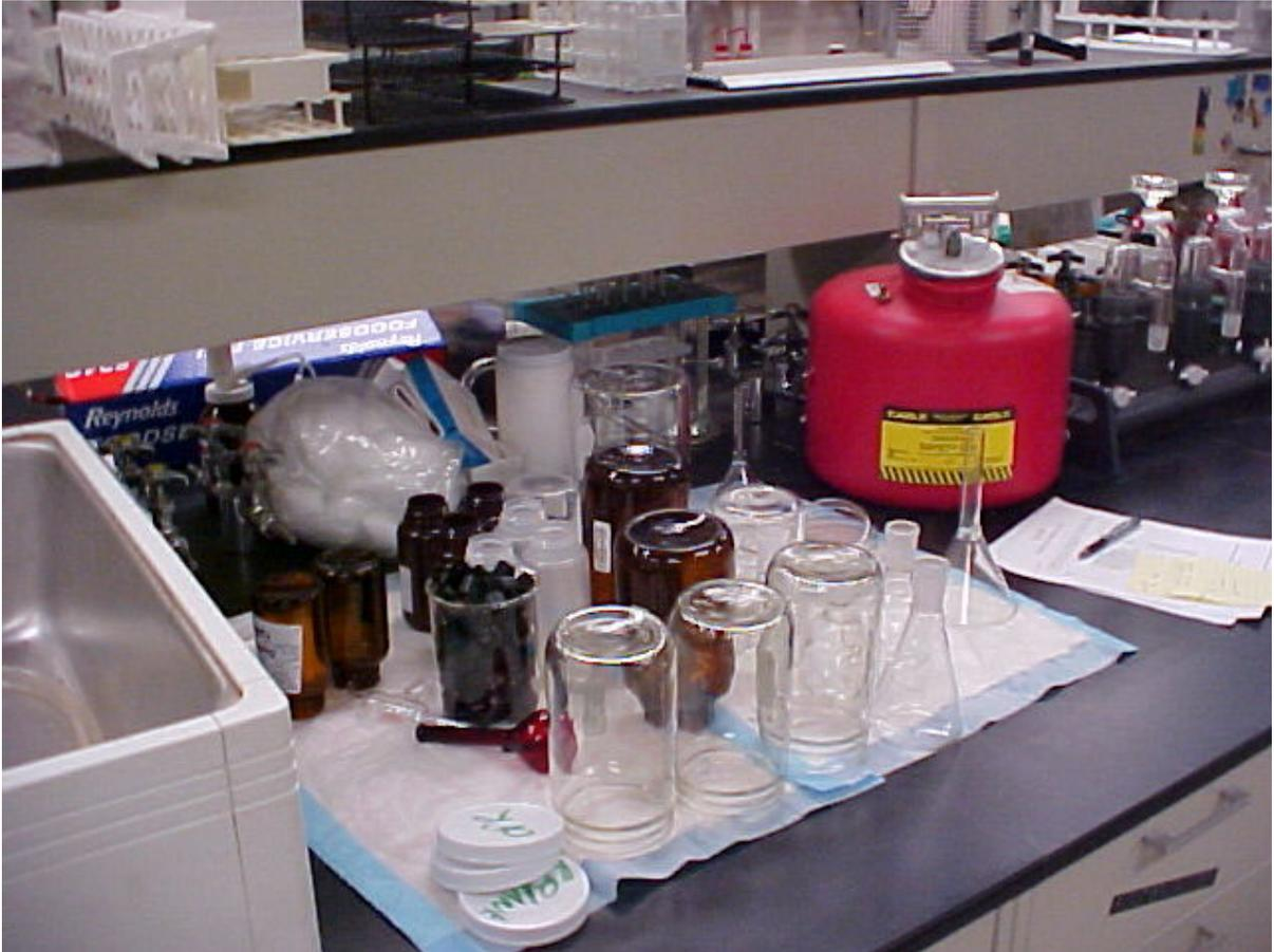
In the above photo, sampling equipment after being washed and being allowed to air dry. You as a Sampler will spend up to 1-2 hours a day preparing your sample bottles. This may include washing your sample tools, bottles and other equipment.
