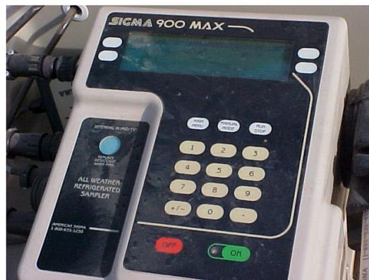
**Tools of the Trade...** Above photos, the Refrigerated Automatic Sampler will have a Data programmer which will allow you to set the time to collect the sample or samples. This machine can also measure the amount of the sample.
