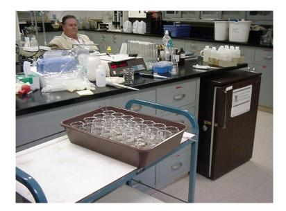
In this photo, the Lab Tech is waiting for the Sampler to return with samples. You can see the small refrigerator with a lock on it. Samplers will normally release the samples to the Chemist, but if the Chemist is out of the office, or after work hours, you will place the samples in the refrigerator and lock it. Write on your chain-of-custody report that you placed the samples in the locked refrigerator.
