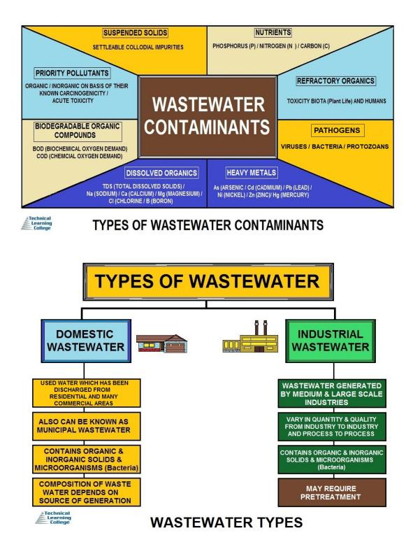
The diagram above shows the difference between domestic wastewater and industrial wastewater
