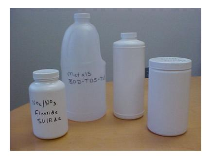
NO<sub>2</sub>/NO<sub>3</sub>, Fluoride, Sulfide, Metals, BOD-TDS-TSS Wide-mouth Sludge/Metals bottle
