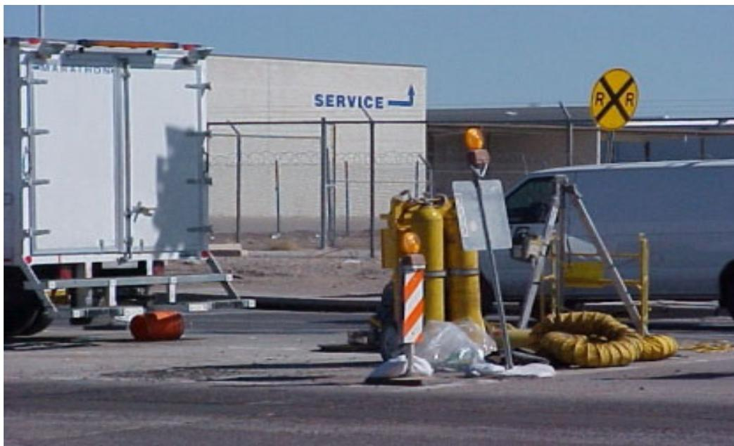
Wastewater sampler set-up in traffic to obtain composite sample from a sewer manhole. Notice the tri-pod and barricades.
