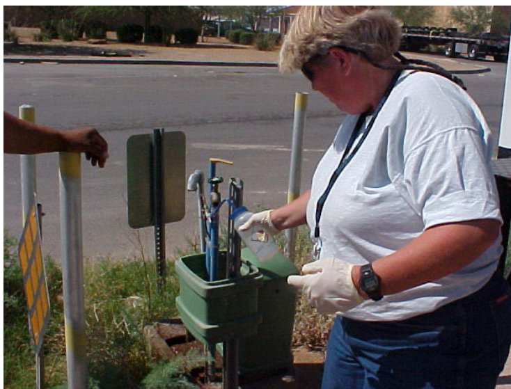
Using alcohol to disinfect a special sample tap before obtaining a sample.
