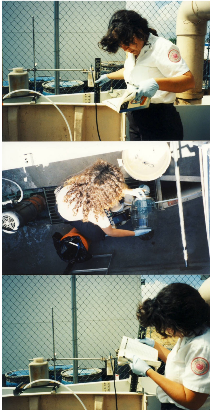
Here is a wastewater Inspector utilizing the auto sampler's manual to help adjust the time and adjust for the correct flow for a composite sample. You can see that she is pouring off the pickle jar.
