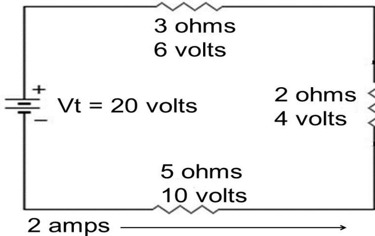
If amps remain the same throughout the circuit then you would have a voltage drop across each load of resistance. This is done by using Ohm's Law. Let's take a close look and see what happens when we take the voltage drops out.
