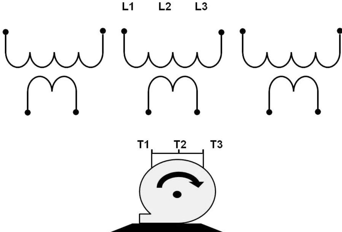
Connect the three transformers in wye-wye, and connect the motor so that it runs in the forward direction, and with no reversed phase polarity.
