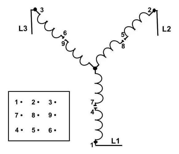
Above is the schematic for a dual voltage wye connected motor, and its terminal board.
