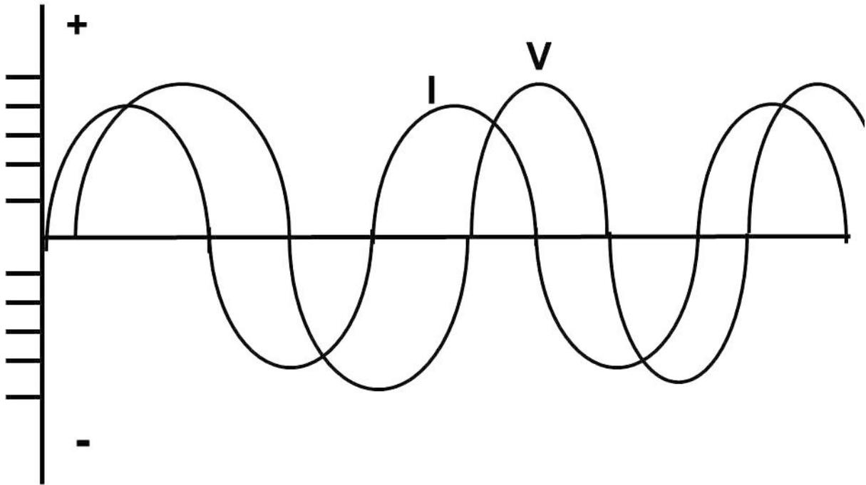
Electromagnetic inductance, as we saw in Lesson 2, is the generation of a voltage whenever current changes its value in a wire. When the wire is coiled, the effect is intensified.
