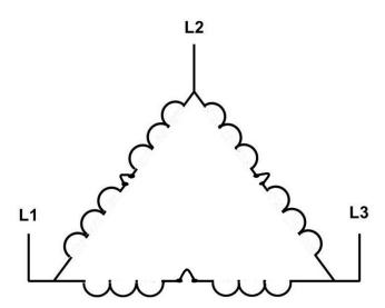
For high voltage, the leads or terminals are jumpered to connect the windings in series, as illustrated in this delta motor.
