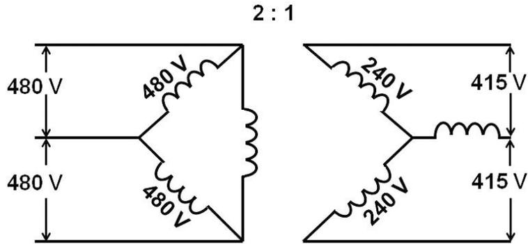
$$V_S = V_P \times \text{TURNS RATIO} \times 1.73$$
