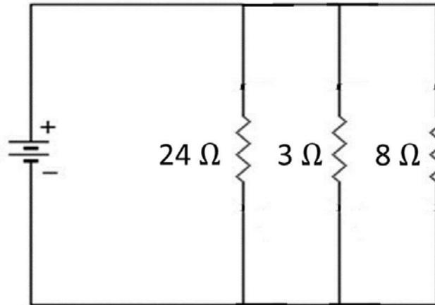
$$R_t \text{ or } R_{eq} = \frac{1}{\frac{1}{R_1} + \frac{1}{R_2} + \frac{1}{R_3} + \dots}$$
