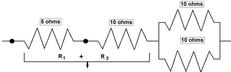
1. First, replace any two components that are connected in series with a single component having a resistance equal to the sum of their resistances. In other words, if you find two components joined together in series, and nothing else is connected to their junction, add their resistances and replace them with a single equivalent component.
