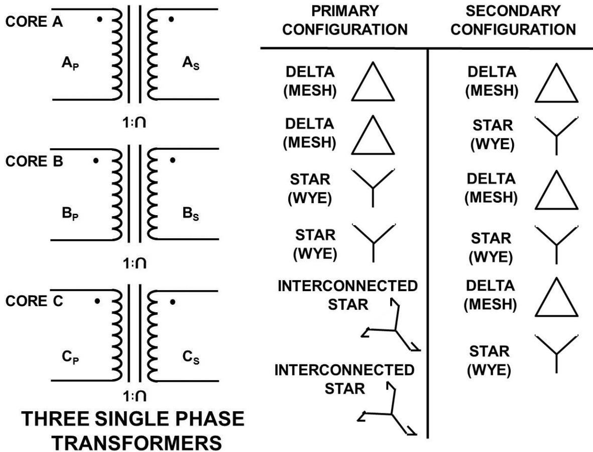
The primary and secondary windings of a transformer can be connected in different configuration as shown to meet practically any requirement. In the case of *three phase transformer* windings, three forms of connection are possible: “star” (wye), “delta” (mesh) and “interconnected-star” (zig-zag).
