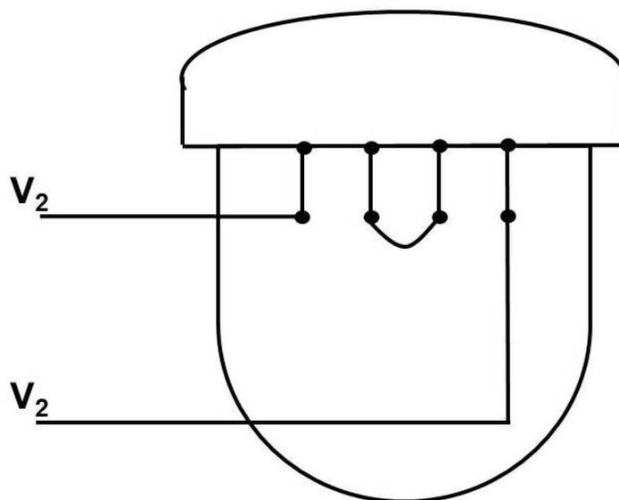
b) If only full voltage loads will be supplied, connect the windings in series.
