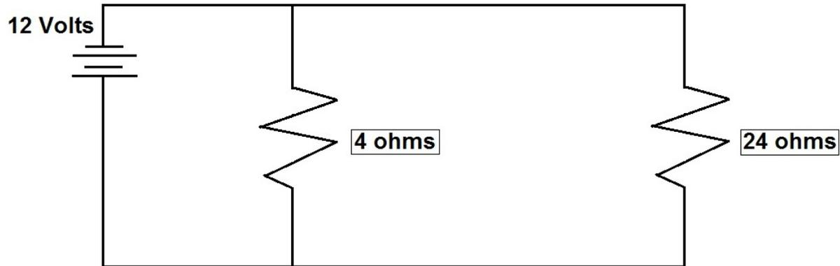
The formula commonly used to calculate the total resistance ( $R_T$ ) of loads wired is
