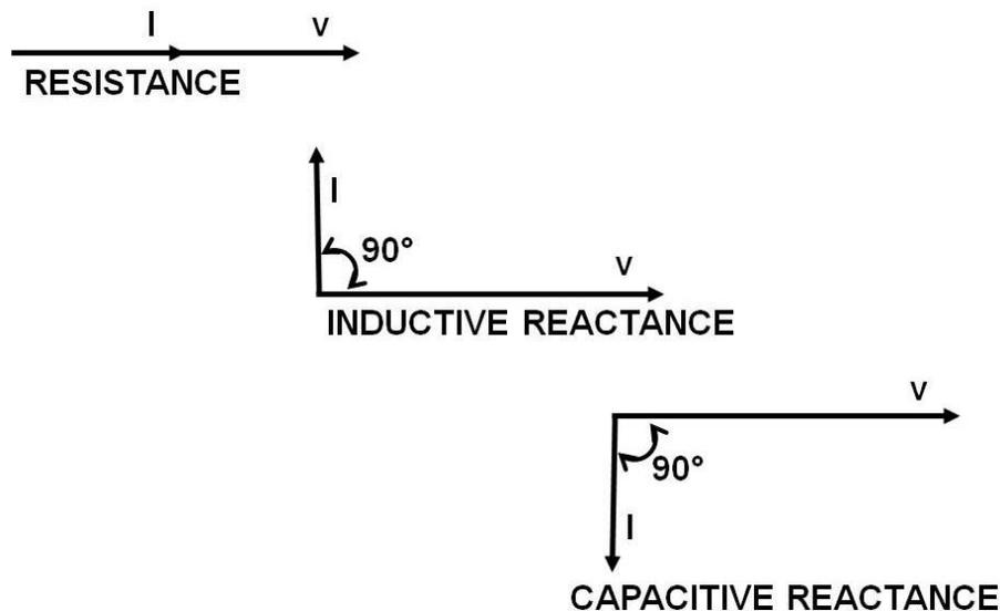
So if the voltage phasor points, like the hand of a clock, at 3:00 o'clock, the current phasor will also point at 3:00.
