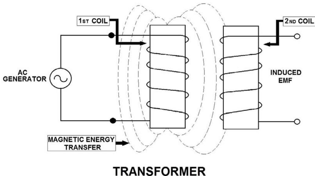
A transformer most commonly consists of two windings of wire wound around a common core to effect tight electromagnetic coupling between the windings. The core material is often a laminated iron core. The coil that receives the electrical input energy is referred to as the primary winding, while the output coil is called the secondary winding.
