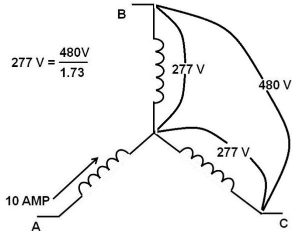
b) In any wye connection, line current and winding current are the same. But line-to-line voltage divides between two windings in wye. The voltage on each winding is line-to-line voltage divided by 1.73.
