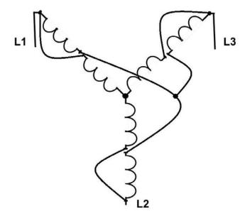
For low voltage, the leads or terminals are jumpered to connect the winding pairs in parallel, as illustrated in this wye motor.
