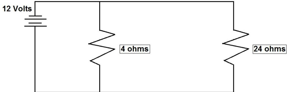
$$R_t = \frac{1}{\frac{1}{R_1} + \frac{1}{R_2} + \frac{1}{R_3} + \dots}$$
