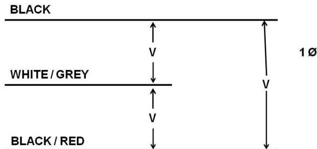
c) If there are two hot conductors and a grounded neutral conductor, single-phase power is available between the hot conductors, and (at a lower voltage) between either hot conductor and the neutral conductor. This is the single-phase 3-wire Edison system.
