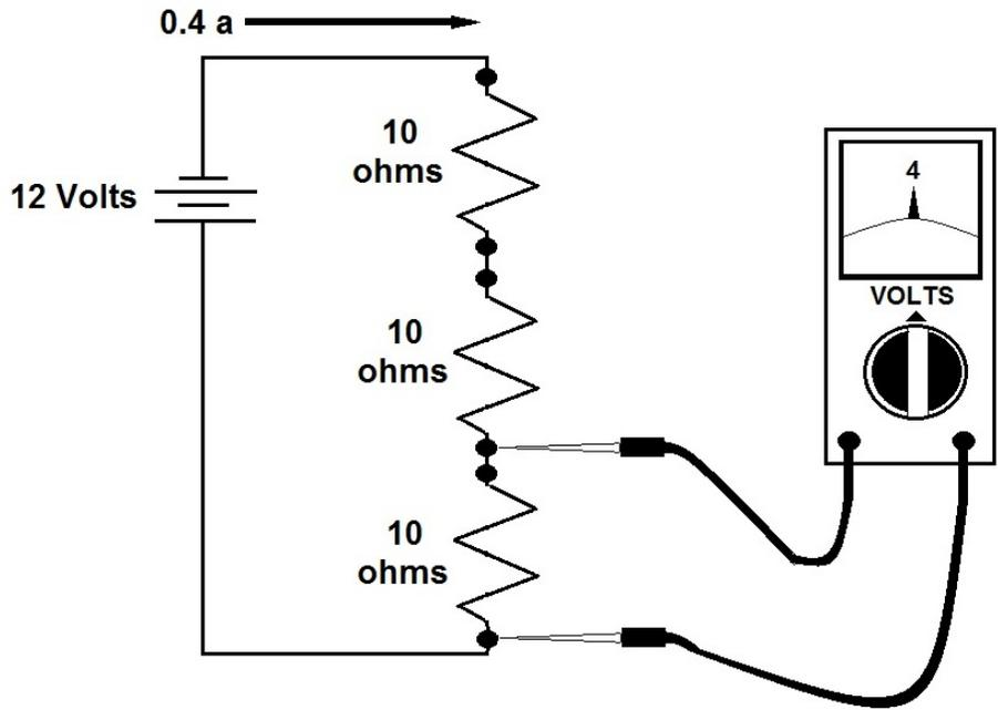
In this example, three 10 ohm loads are connected in series. The total resistance of the circuit is  $10 + 10 + 10 = 30$  ohms.
