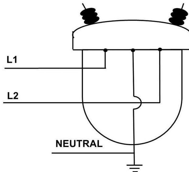
**Secondary.** If a secondary winding has three terminals, the middle one is probably a center tap on the winding.
