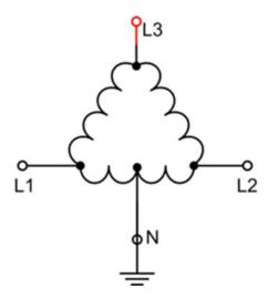
A transformer for a high-leg delta system; 200 V 3-phase motors would be connected to L1, L2 and L3. 200 V Single-phase load would be connected L1 and L2. Single phase 100 V load between either L1 or L2 and neutral (N). L3 (wild or high leg) will be 173.2 V to neutral.
