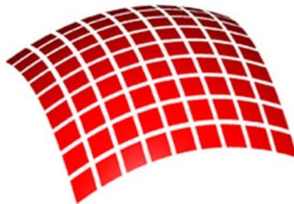
The definition of surface integral relies on splitting the surface  $\Sigma$  into small surface elements. Each element is associated with a vector  $d\mathbf{A}$  of magnitude equal to the area of the element and with direction normal to the element and pointing "outward" (with respect to the orientation of the surface).
