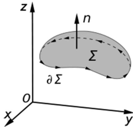
An illustration of Kelvin-Stokes theorem with surface  $\Sigma$  its boundary  $\partial\Sigma$  and orientation  $\mathbf{n}$  set by the right-hand rule.
