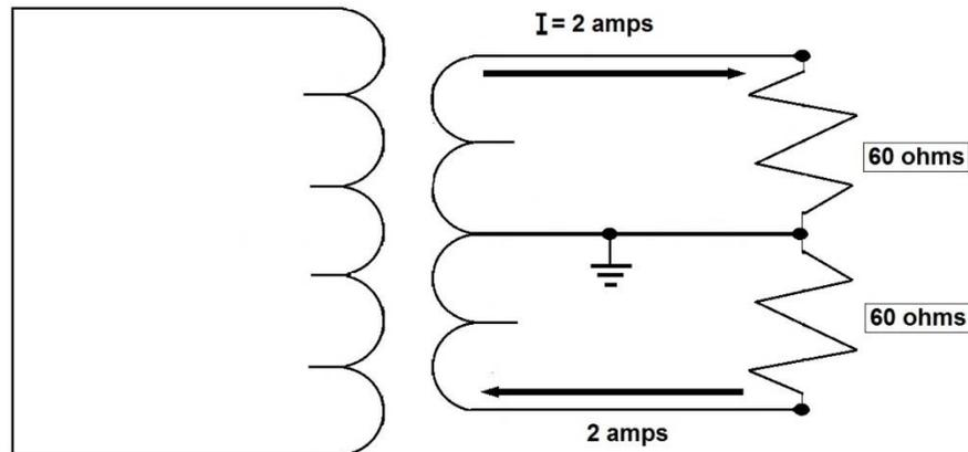
A main advantage of the Edison system is that full line-to-line voltage is available for large power consuming appliances and equipment, but voltage to ground is only half line-to-line voltage. The lower the voltage to ground in any electrical system, the less likely are shorts, fires, and shocks.
