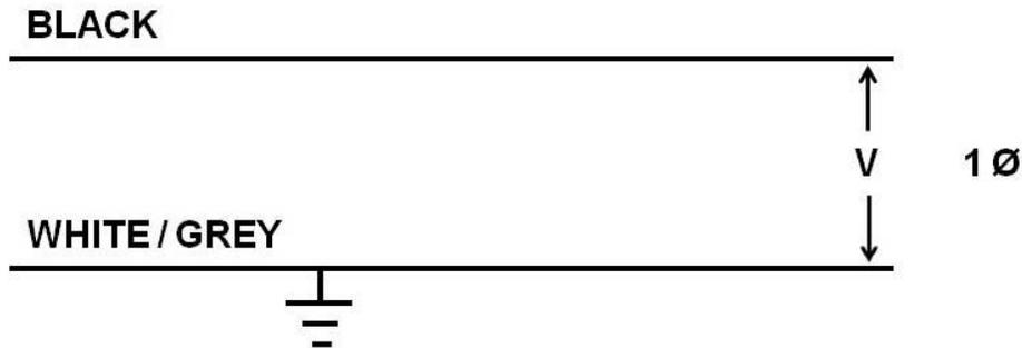
a) If there is only one hot conductor (usually black) and + one grounded conductor (white or grey), single- phase power is available between them.
