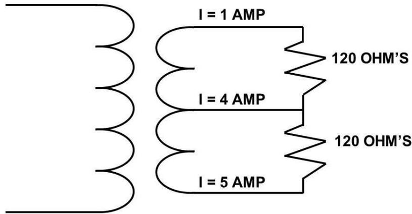
When loads are not balanced-the resistance of one is greater than the other- current flows in the neutral. The neutral carries the difference between the current in the first load and the current in the second load.
