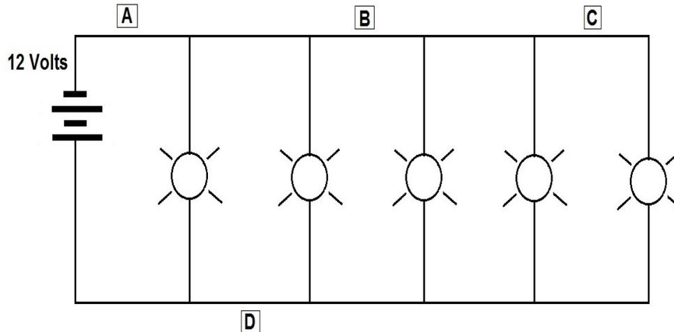
A 12-volt battery supplies five 4-watt indicator lights in parallel. What is the current at points A, B, C, and D when all the lights are on?
