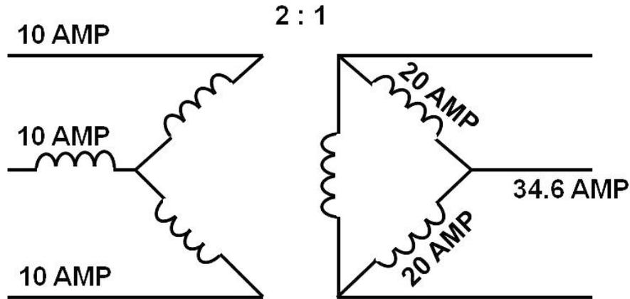
$$I_S = I_P \div \text{TURNS RATIO} \times 1.73$$
