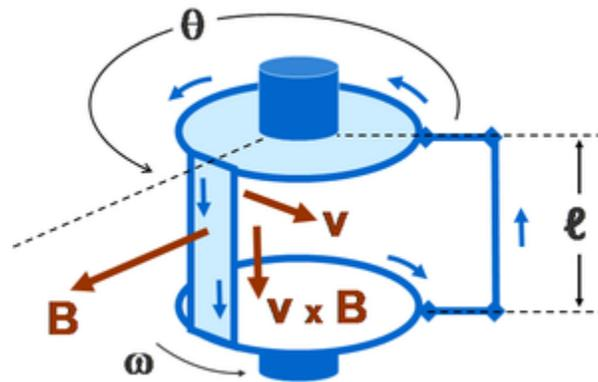
Rectangular wire loop rotating at angular velocity  $\omega$  in radially outward pointing magnetic field  $\mathbf{B}$  of fixed magnitude. The circuit is completed by brushes making sliding contact with top and bottom discs, which have conducting rims. This is a simplified version of the *drum generator*.
