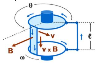
Rectangular wire loop rotating at angular velocity  $\omega$  in radially outward pointing magnetic field **B** of fixed magnitude. The circuit is completed by brushes making sliding contact with top and bottom discs, which have conducting rims. This is a simplified version of the *drum generator*.
