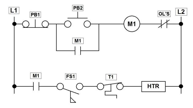
In the circuit above, the blower motor runs but the heater does not work. What would you test first?
