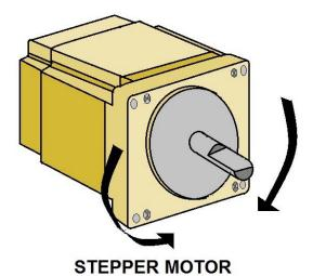
Brushless, Synchronous Electric Motor that coverts digital pulses into shaft rotations
