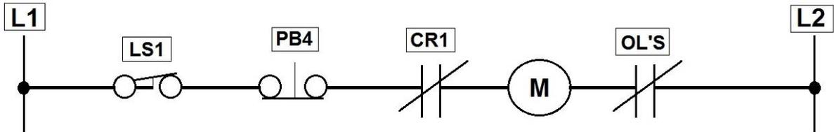
1. Control voltage is 120 volts. Assume that an overload on the motor has tripped. What voltage would you expect to find across coil M (point A to point 8) in this circuit? What would points A and B read to ground?
