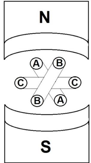
As the coils turn through the magnetic field, power is sent out on three lines. Three current and voltage sine waves are generated, 120 degrees out of phase with each other. Each sine wave represents the current or voltage on one of the phases.
