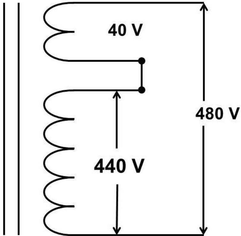
If, for example, the local-supply lines provide 440 volts, but a new motor is rated at 480, a buck/boost transformer would be connected as in A.
