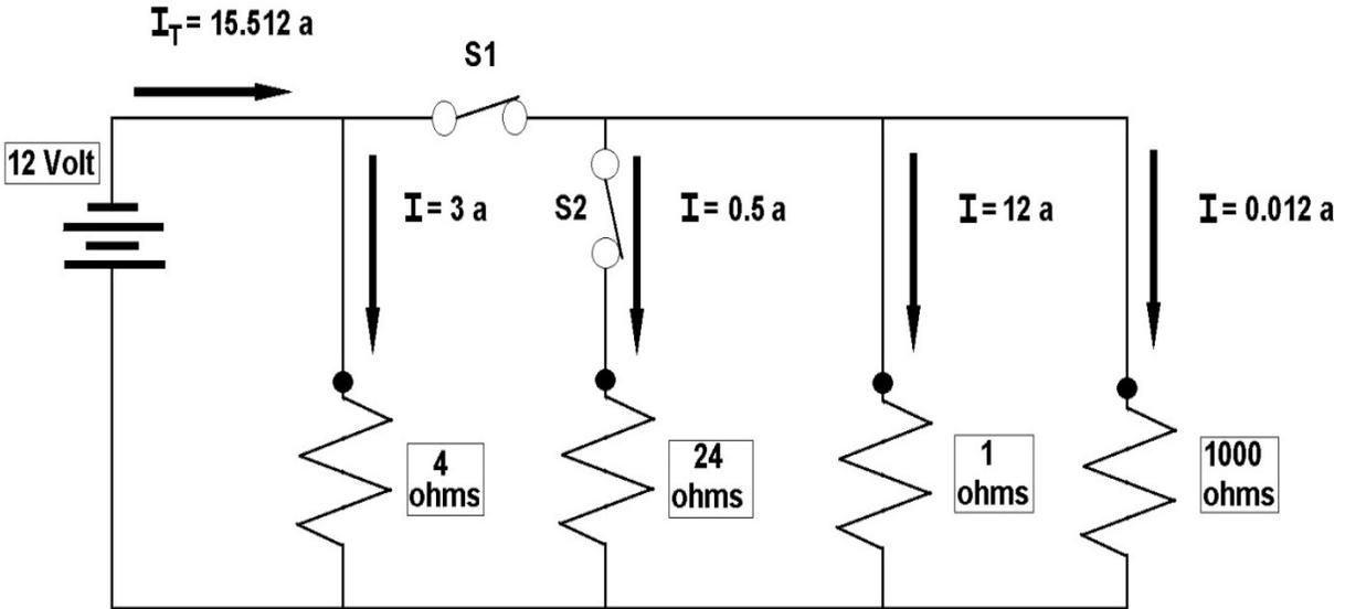
A. Suppose a 1 ohm load and a 1000 ohm load are added in parallel with the 4 ohm and the 24 ohm loads. The current in the 1 ohm load will be  $12 \text{ volts}/1 \text{ ohm} = 12 \text{ amperes}$ . The current in the 1000 ohm load will be  $12 \text{ volts}/1000 \text{ ohms} = 0.012 \text{ amperes}$ . The total circuit current will now be  $3 + 0.5 + 12 + 0.012 = 15.512 \text{ amperes}$ .
