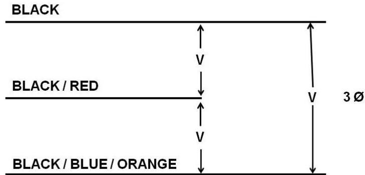
d) If there are three hot conductors, the source is three-phase. Single-phase power is available between any two of the conductors. Connection of three-phase loads to all three hot conductors provides three-phase power. Voltage between each pair of conductors should measure the same, but the voltages will be 120 degrees out of phase.
