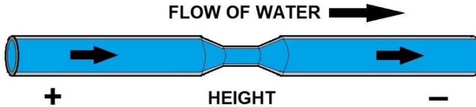
**Electricity flow can be compared to flow of water:**
