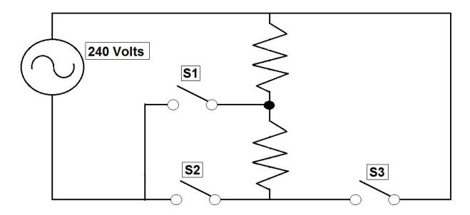
Two oven elements are arranged with three switches to provide three heat settings: high, medium, and low. In low, the two elements are connected in series between 240 volts. In medium, one is connected to 240 volts and the other is not connected. In high, both elements are connected across 240 volts in parallel.
