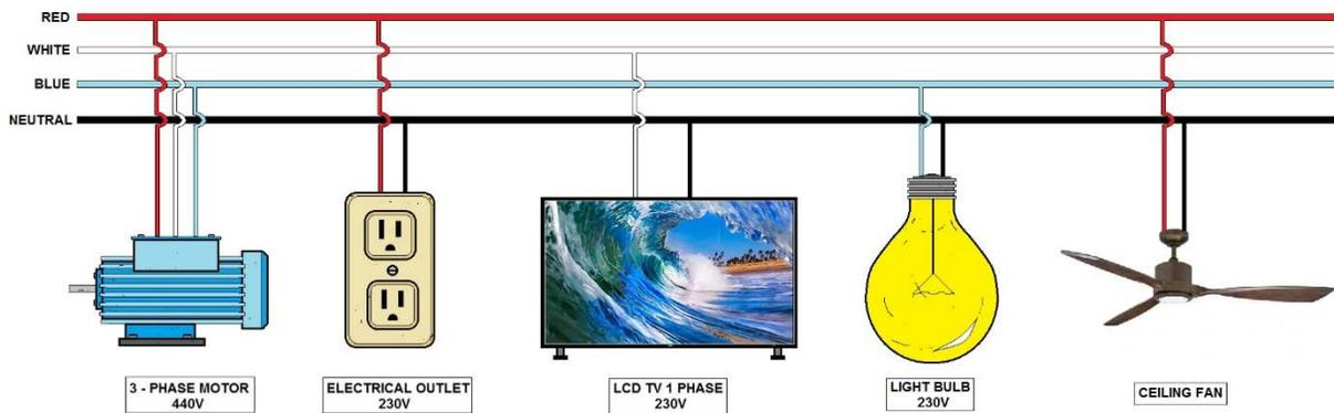
SINGLE PHASE or 3 PHASE LOADS IN A 3 PHASE WIRING DISTRIBUTION SYSTEM
