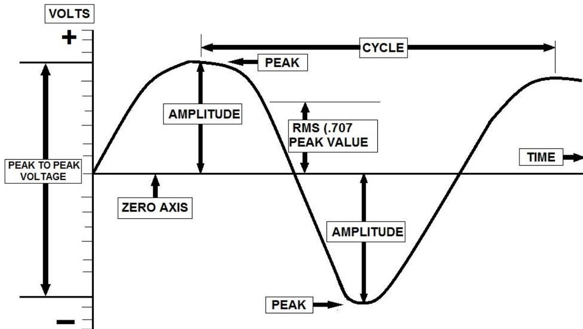
Alternating voltage and current generated by rotary motion take the form of a sine wave. It is the most common form of alternating current and voltage. As the conductor turns through the magnetic field, it cuts through the magnetic lines of force at a varying rate. As a result, voltage varies in a regular, repetitive pattern.
