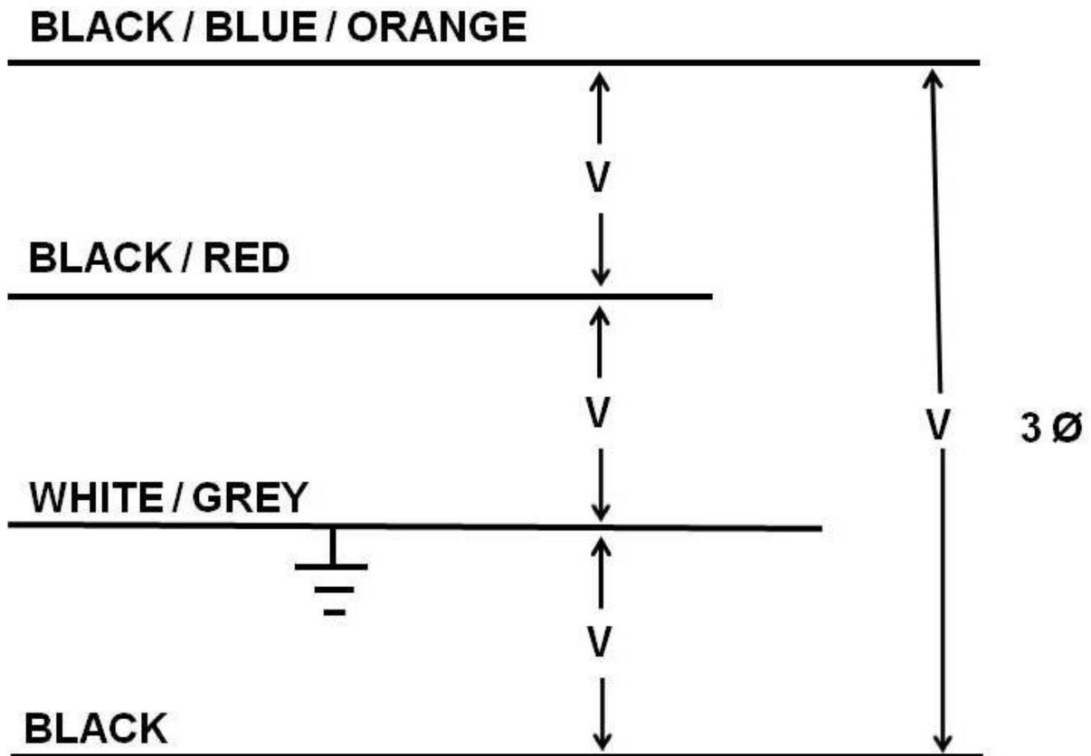
e) If there are three hot conductors and a grounded neutral conductor, single phase power is also available between two or three of the hot conductors and the neutral. This is a 4-wire three-phase system.
