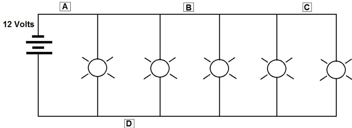
(The above is a Parallel circuit not a Series circuit.)
