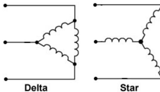
The most common connections are Y-A, A-Y, A-A and Y-Y.
