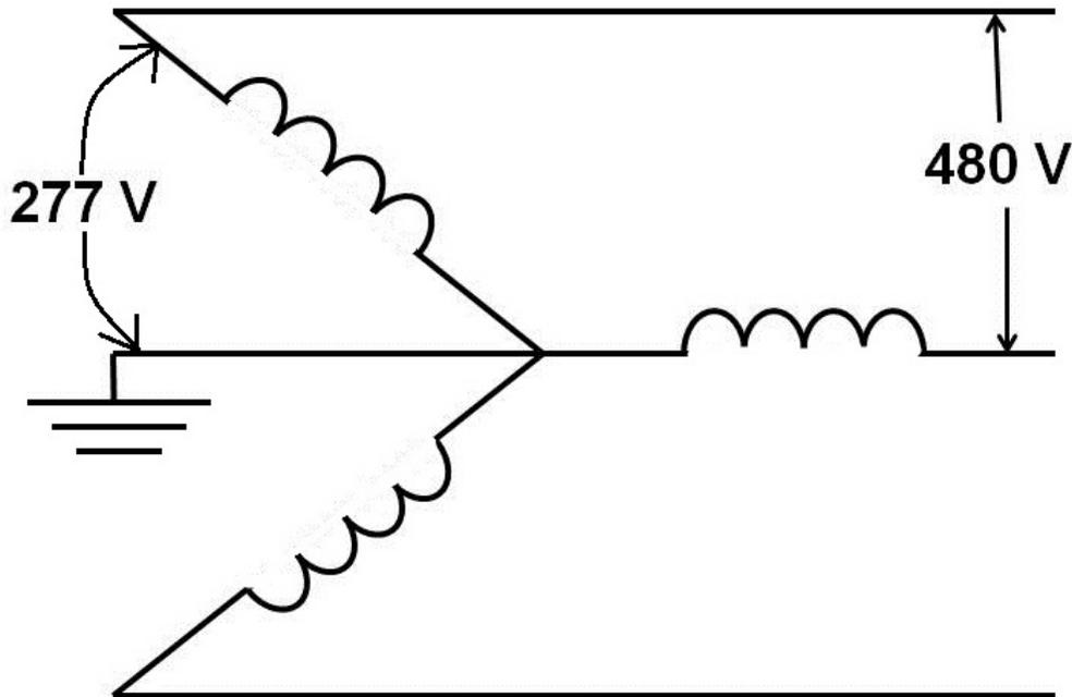
Neutral junctions of wye' connected transformer windings, both primary and secondary, are usually grounded. As a result, the voltages to ground on power lines in a wye system will be equal to line-to-line voltage divided by 1.73. Line-to-line voltage will be equal to line-to-ground voltage times 1.73. If voltages are different from this on any power line, something is wrong.
