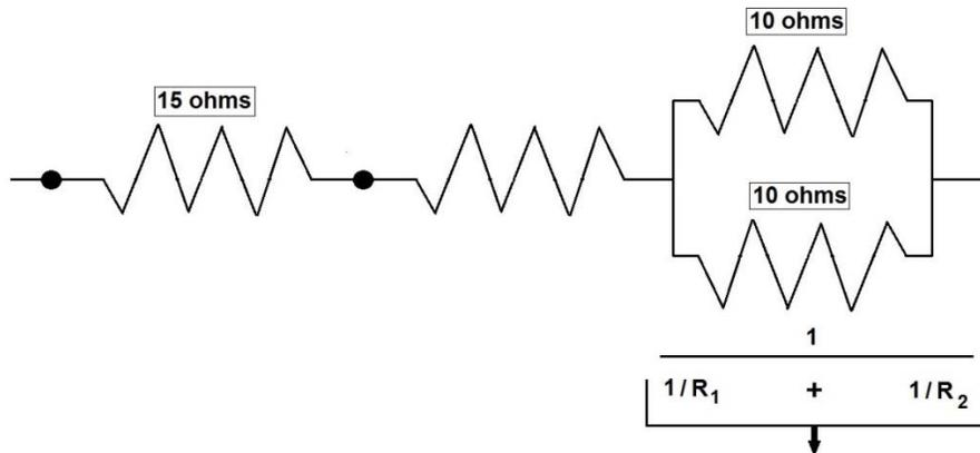
2. Second, replace any two components that are connected in parallel with a single component having a conductance equal to the sum of their conductances. You will need to convert the equivalent conductance back into a resistance before adding it to the resistance of another component in series.
