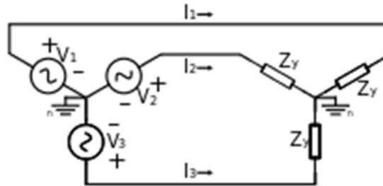
Three phase AC generator connected as a wye source to a wye connected load.
