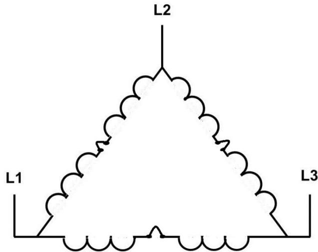
For high voltage, the leads or terminals are jumpered to connect the windings in series, as illustrated in this delta motor.
