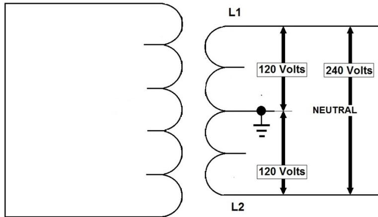
Most single-phase AC is supplied from a 3-wire EDISON SYSTEM. There are two hot conductors, and one grounded neutral conductor. In a 120/240 volt system, the voltage between each hot wire and neutral is 120 volts. Voltage between the two hot wires is 240 volts. In a 240/480 volt system, available voltages are 240 volts and 480 volts.
