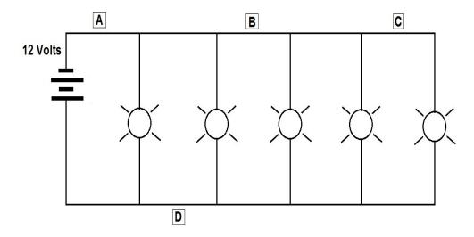
A 12-volt battery supplies five 4-watt indicator lights in parallel. What is the current at points A, B, C, and 0 when all the lights are on?
