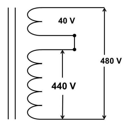
If, for example, the local-supply lines provide 440 volts, but a new motor is rated at 480, a buck/boost transformer would be connected as in A.
