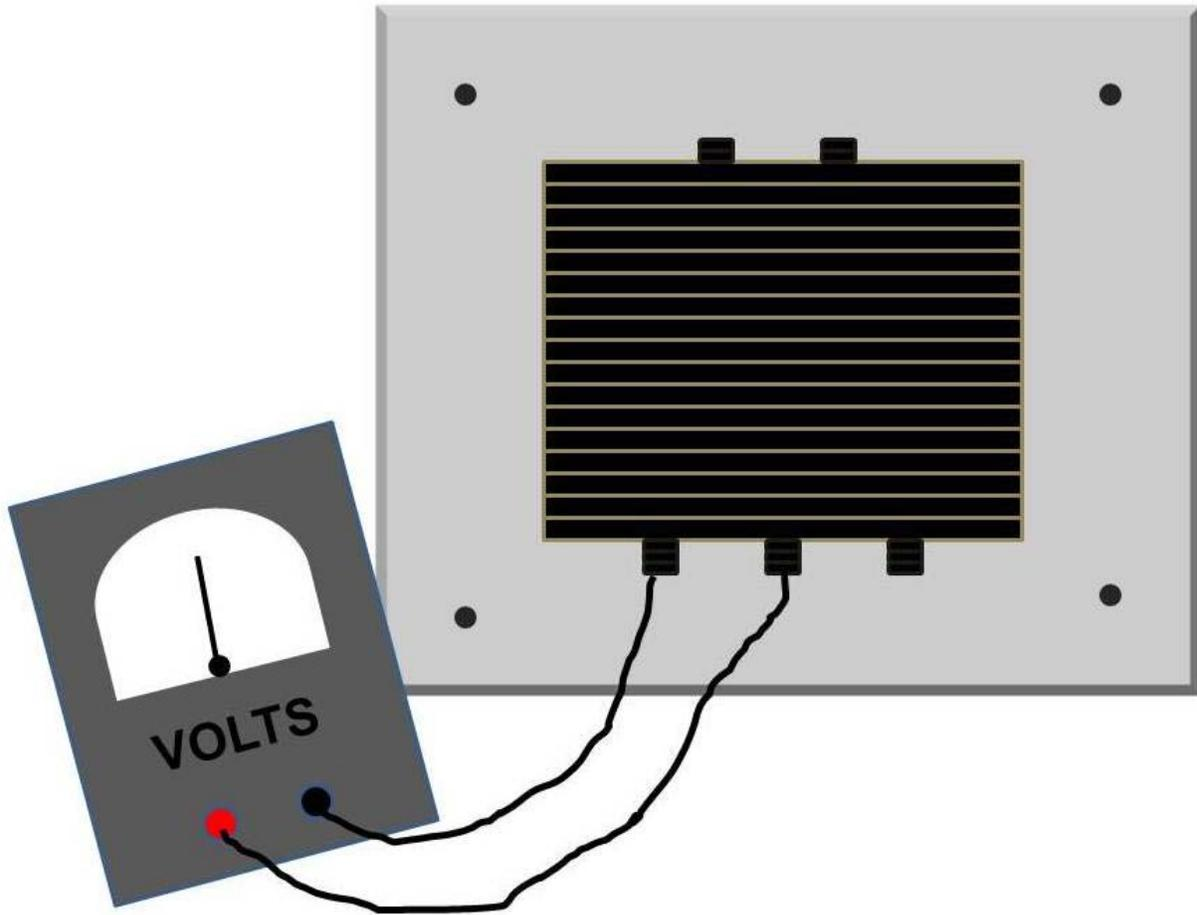
If the secondary has three terminals, and you are not sure which one is the center tap, apply a test voltage to the primary and measure the voltage between secondary terminal pairs. The center tap terminal will read half voltage to either of the others.
