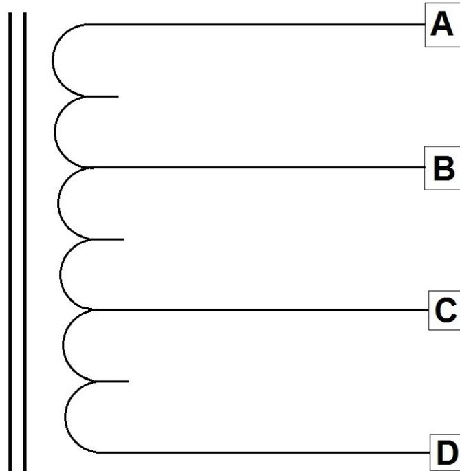
The autotransformer shown above has two taps, equally spaced on the winding. At which points should the primary and secondary connections be made to:
