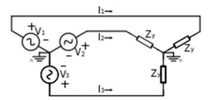
Three phase AC generator connected as a wye source to a wye connected load.
