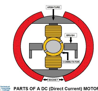
**PARTS OF A DC (Direct Current) MOTOR**
