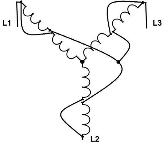
For low voltage, the leads or terminals are jumpered to connect the winding pairs in parallel, as illustrated in this wye motor.
