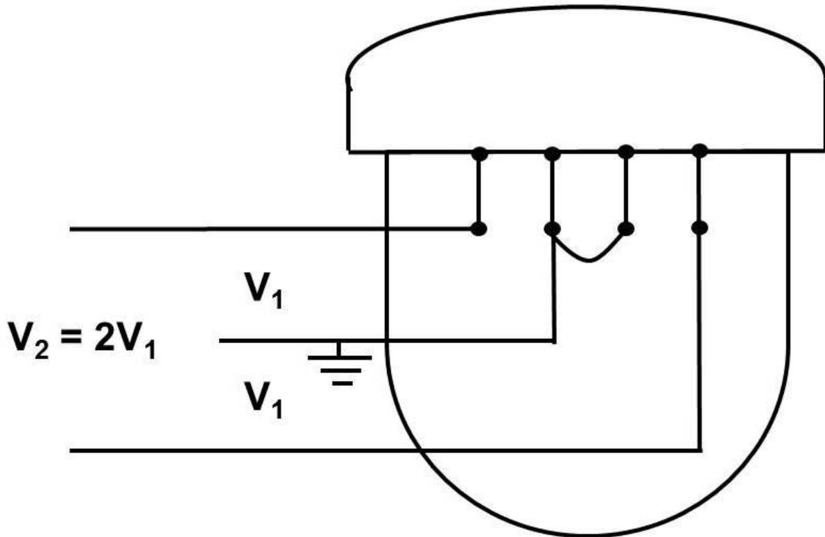
c) If both half voltage and full voltage loads will be supplied, connect the windings in series and add a grounded neutral conductor to the junction of the windings.
