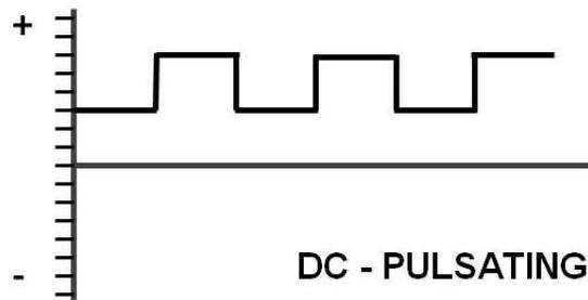
Pulsating DC does change in magnitude. But it also always appears on the same side of the zero axis on an oscilloscope, because its polarity is constant.
