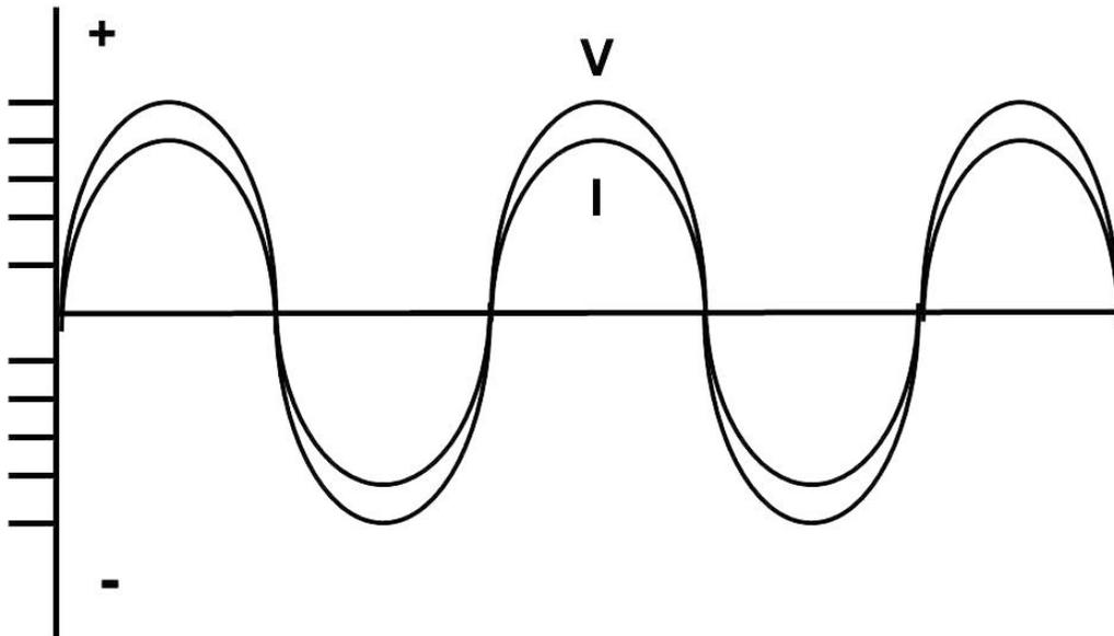
Both current and voltage follow a sine wave pattern, with the positive and negative voltage and current peaks occurring at exactly the same time.
