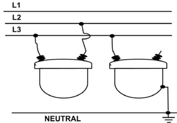
**Primary.** Single-phase transformers with two primary terminals or leads insulated for high voltage may be connected between two hot conductors or between a hot conductor and neutral.
