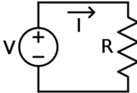
An electric circuit is an interconnection of electric components such that electric charge is made to flow along a closed path (a circuit), usually to perform some useful task.
