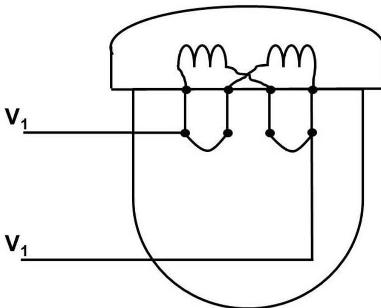
a) If only half voltage loads will be supplied, connect the secondary windings in parallel.
