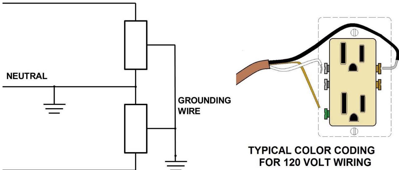
For example, the neutral in a 3-wire Edison system is a grounded conductor, because it is normally expected to carry load current whenever the loads are unbalanced. It should not normally be used to ground parts or equipment. If resistance developed in its connections, anything connected to ground by it would have voltage on it.
