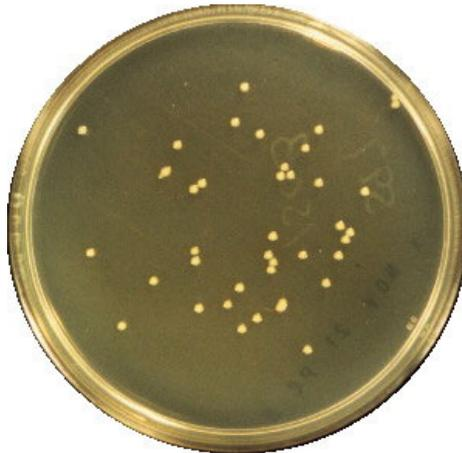
Top photograph, HPC plate. Bottom, Bac-T or Colilert samples, the yellow indicates coliform bacteria, if this sample fluoresces under a black light that means that fecal or e. coli is present.
