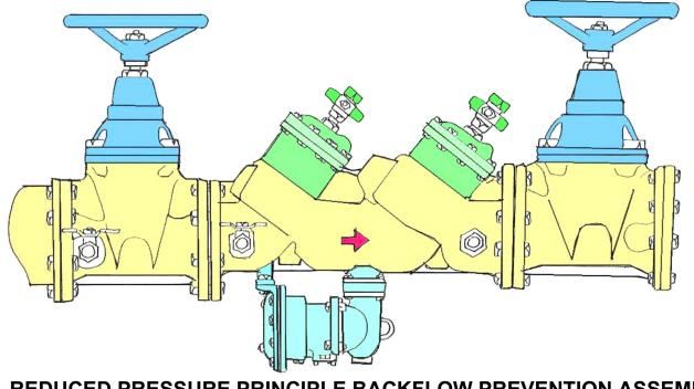
REDUCED PRESSURE PRINCIPLE BACKFLOW PREVENTION ASSEMBLY (RP)
