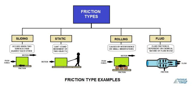
Friction is the force resisting the relative motion of solid surfaces, fluid layers, and material elements sliding against each other.
