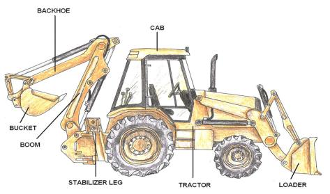
Backhoes are one of the most common types of construction equipment found today. And rightly so as their versatility and maneuverability makes the back hoe the equipment of choice for most construction jobs. Backhoe loaders can dig, scrape, load material, lift and with specialized attachments do almost any required task. No one should operate a back hoe unless specifically trained and authorized by the company.
