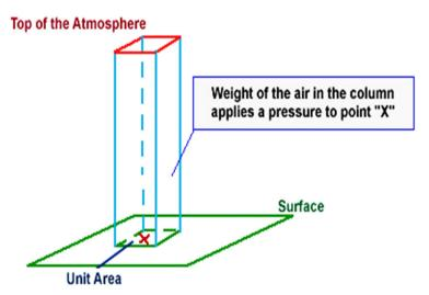
In the diagram, the pressure at point "X" increases as the weight of the air above it increases. The same can be said about decreasing pressure, where the pressure at point "X" decreases if the weight of the air above it also decreases.
