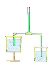
If the levels in the two basins are not equal, fluid flows from the **PASCAL'S SIPHON** basin with the higher level into the one with the lower level, until the levels are equal.
