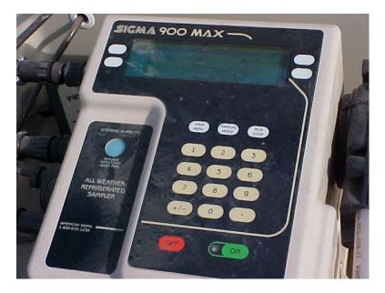
The Refrigerated Automatic Sampler will have a Data programmer that will allow you to set the time to collect the sample or samples. This machine can also measure the amount of the sample. These can also be used for the collection of composite samples. Sometimes you will see a pH probe with real-time readings sent to the Operator's Command Center. This is a common sight for most wastewater plants and SIUs.
