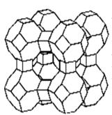
The basic building blocks of zeolites are tetrahedral consisting of four oxygen anions and one centrally positioned silicon or aluminum cation. Zeolites are classified according to the various tetrahedral frameworks formed by these basic building blocks. The structure of the synthetic zeolites of types A, X and Y which have gained importance in industrial processes, are shown in the figure.
