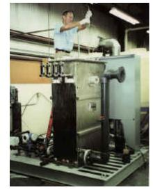
This 10 gpm reactor is used to demonstrate the oxidation of arsenic in a small town's water supply in Northern California. After oxidation, the arsenic was removed with iron hydroxide to produce clean water which contained less arsenic than the new stringent health limits.
