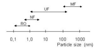
The smaller the pore size of the membranes, the higher the pressure needed to achieve separation. In the case of microfiltration and ultrafiltration we speak of low pressure processes, while nanofiltration and reverse osmosis are high pressure processes.
