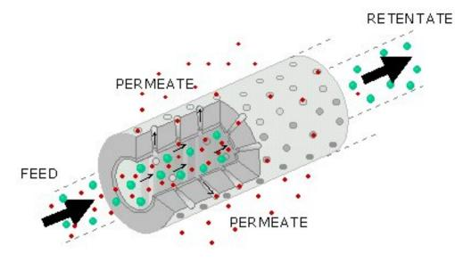
Transport through the membrane is performed by a pressure difference, a concentration difference, a chemical or electrical potential difference as a driving force. The membrane itself forms a semi-permeable barrier through which some particles are transported faster than others, so that a separation occurs.
