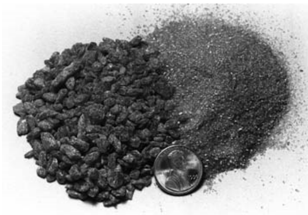
Figure 1. Copper sulfate is available as nuggets (left) or as finely ground crystals.
