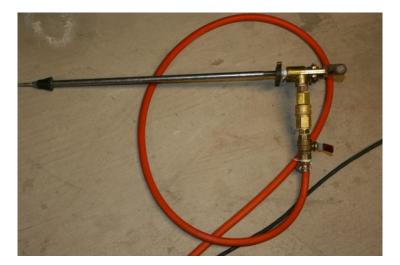
Using a subslab injector, inject insecticide through holes at the rate of 4 gallons per 10 linear feet. After application, plug all holes with mortar or any other special compound.
